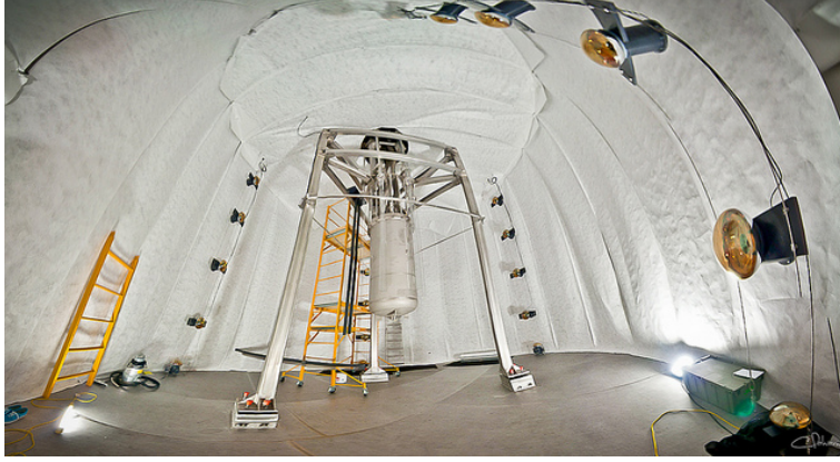
Figure 2.11: Inside the water tank of the LUX detector. 20 large PMTs are installed for veto. Taken from Ref. [10].
