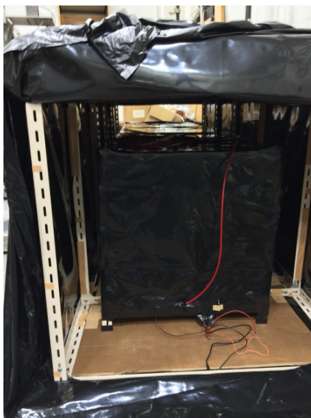
Figure 5.22: The outer light-tight box and the apparatus. After the installation of instruments, both ends of the outer box were closed.
