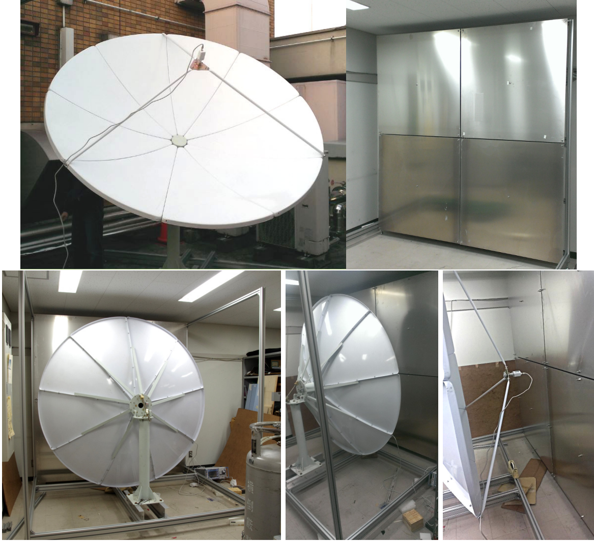
Figure 4.4: Photographs of the set-up of the experiment described in Ref. [27, 28, 29]. (upper left) Parabolic dish of 2.2 m diameter and 77 cm focal length. (upper right) Plane reflector made out of four aluminum plates of 1.2 m (height) \times 1.2 m (width) \times 2 mm (thickness). (bottom) Combination of the dish and the plane reflector.
