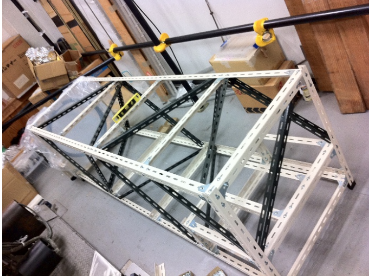
Figure 5.10: Photograph of the reinforced version of the framework. It also has a platform to mount optical instruments.
