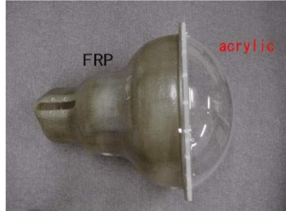
Figure 3.4: Left: The schematic view of the 20-inch PMT [58]. Right: The picture of the FRP and the acrylic case for PMT.
