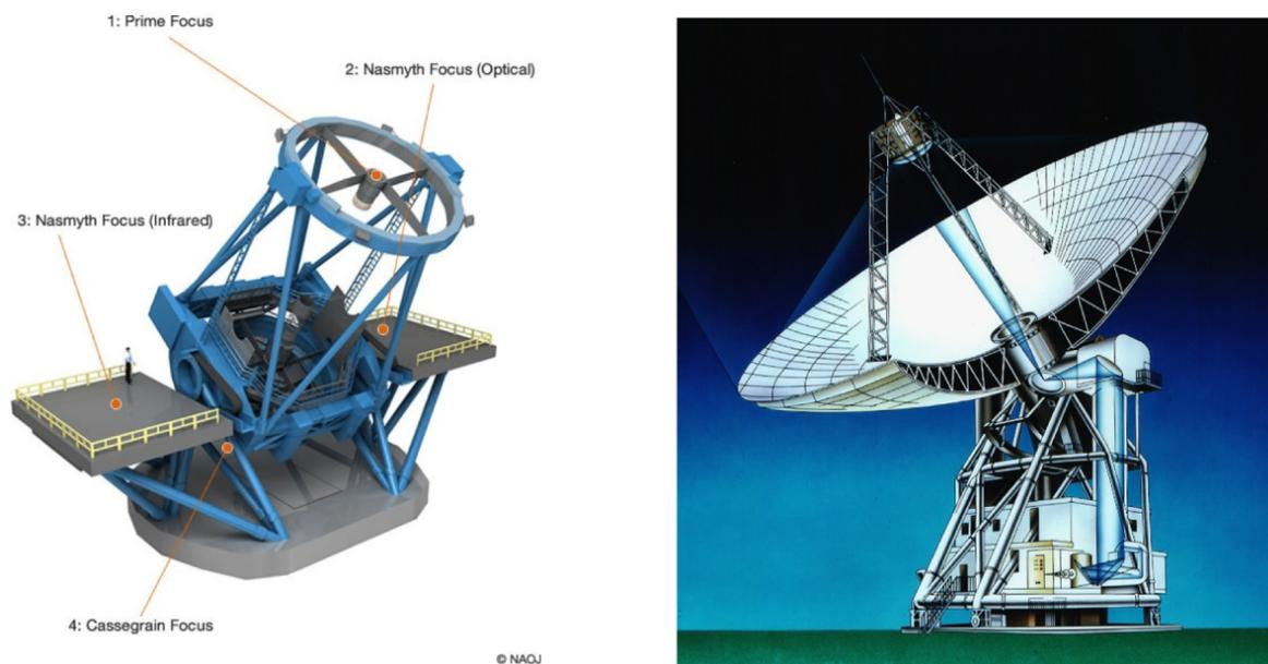
Figure 2.1: *Left*: Image of the Subaru 8.2 m telescope. This figure is reproduced from <http://subarutelescope.org/Introduction/telescope.html>. *Right*: Image of the Nobeyama 45 m radio telescope. This figure is reproduced from <http://www.nro.nao.ac.jp/~nro45mrt/html/pictures/illust/index-e.html>.
