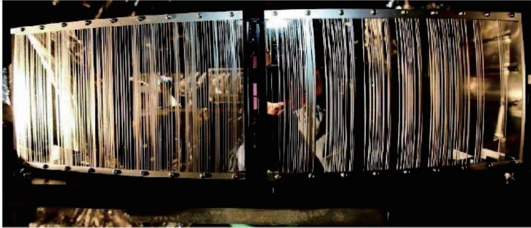
Figure 3.4: The mask mirror of IRS1 spectrograph. From Kimura et al. (2010).
