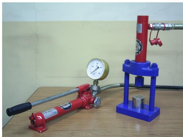
Figure 2–3. Photograph of hydraulic press.
