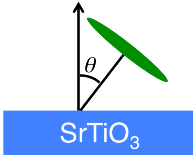
Figure 4.15 A schematic image for representing orientation angle \theta . A green ellipse represents the phthalocyanine molecule.
