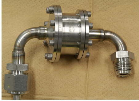
Figure 7.1: The cryogenic precision burst disc from Hydrodyne. It works at 5 K and protects the X-ray window from overpressure.
