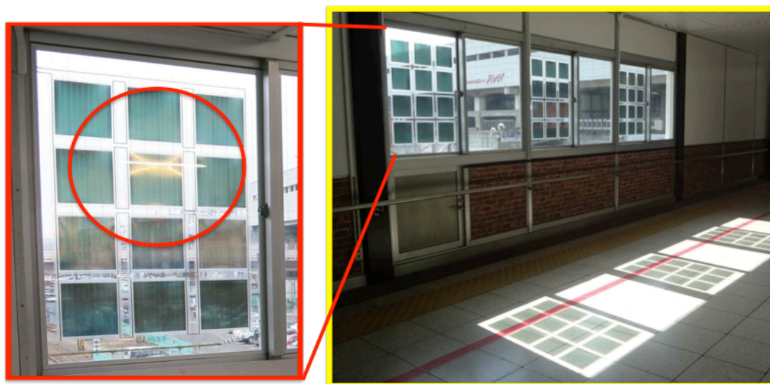
Figure 1. A real window application of transparent OSCs (right) and the highlighted problem of sunlight glare from use of reflective (left) Ag even when thin metal electrodes were used.
