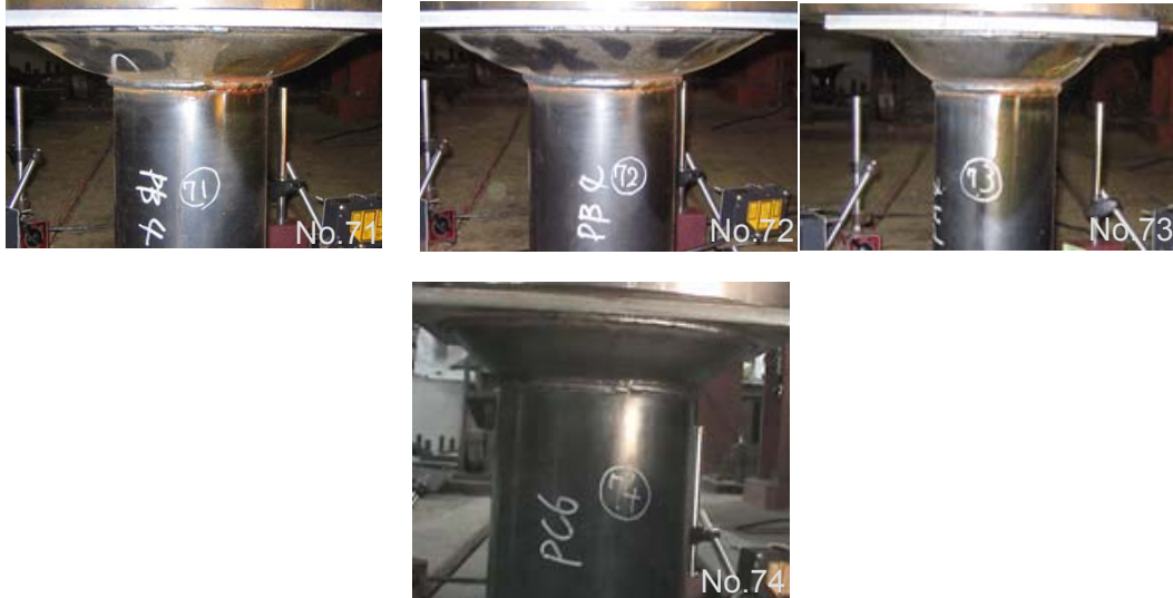
(a) Specimens with joint region failure
