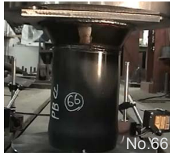
(b) Specimen with elephant foot buckling of cylindrical wall
