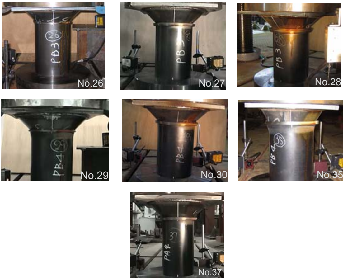
(a) Specimens with tapered ring failure
