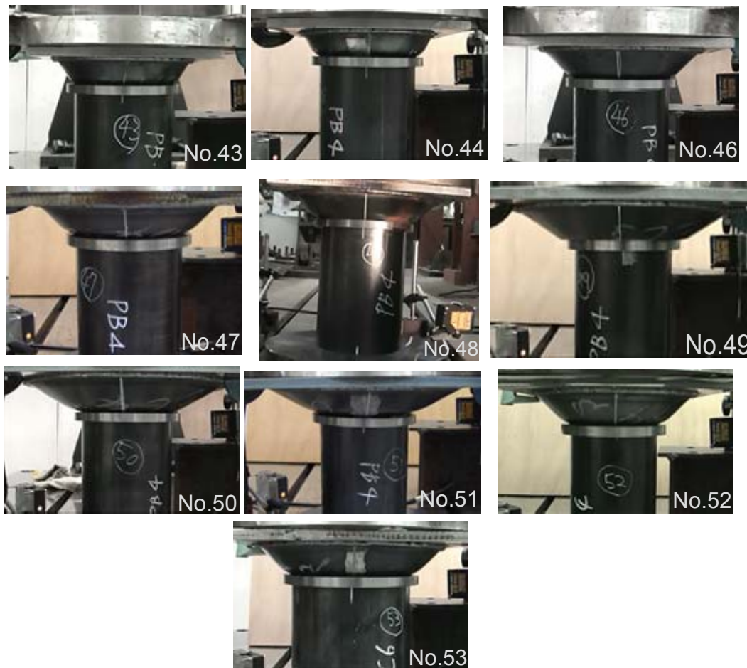
(a) Specimens with conical wall failure
