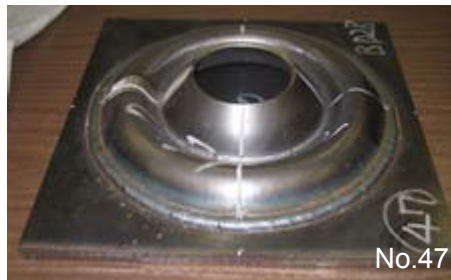
Fig. 2-19 Deformation of conical wall after testing in specimen No. 47
