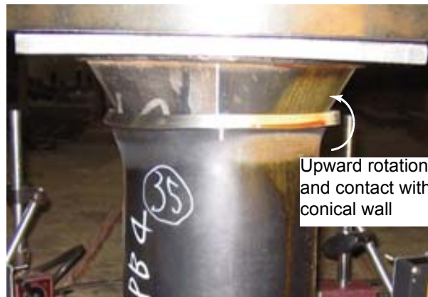
Fig. 4-7 Ultimate behavior of tapered ring in experimental specimen No. 35
