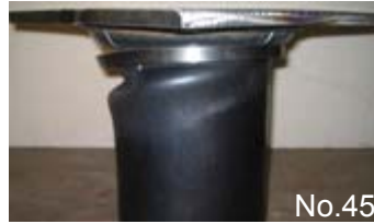
(b) Specimen with asymmetric failure mode
