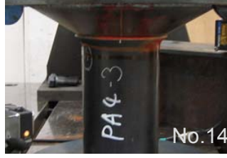
(a) Specimens with cylinder edge failure
