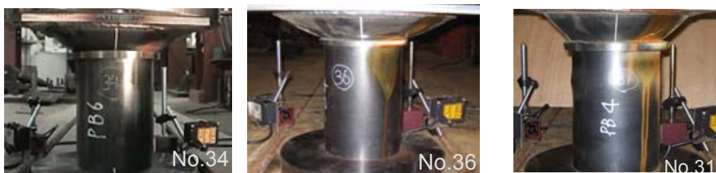
(a) Specimens with tapered ring failure
