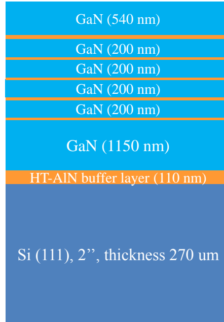
Figure A.2 GaN sample grown on silicon by MOCVD.
