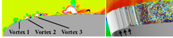
(a) Vortex 1, 2, and 3 on phase-averaged field (left) and instantaneous field (right) at \phi/2\pi = 1/10
