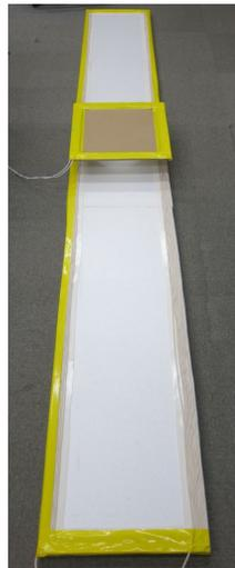
Figure 4.3: Fabricated three-meter coil and receiver coil.
