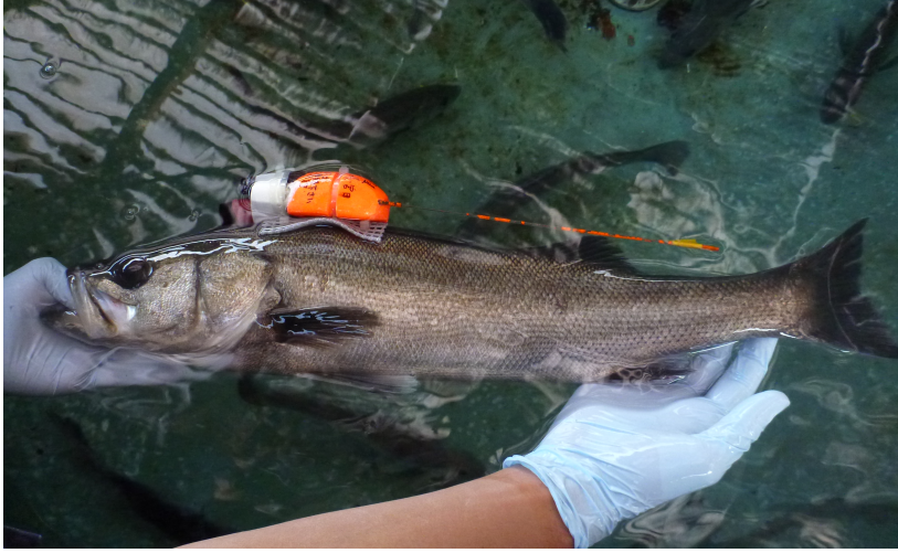
Fig. 4-2 Japanese sea bass attached the tag package composed with three-axis accelerometer, video logger, VHF transmitter, and float
