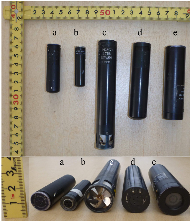
Fig. 4-1 Five different types of data-logger attached to Japanese sea bass in field study. Accelerometers ( a : two-axis, b : three-axis, and c : three-axis acceleration with speed sensor), d : conductivity (salinity), and e : video recorder, respectively
