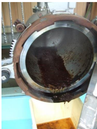
Fig. 4.3 Pulps and black liquor after steam explosion in the receiver.
