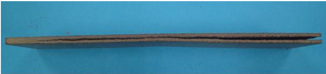
Fig. 2.6 The side-view of the exfoliated board (Length of side: 30cm; Thickness: 5mm).
