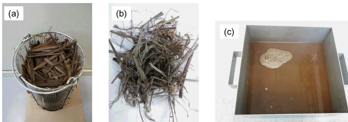
Fig. 4.26 Steam treatment products. (a) Steam treated wet rice straw. (b) Steam treated rice straw after over-dry. (c) Drainage of steam treatment.
