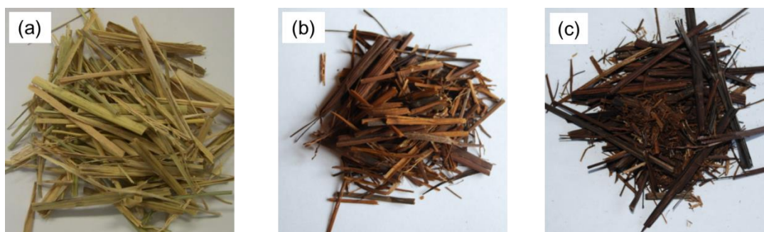
Fig. 4.15 Heat treated rice straw chip ( \leq 50\text{mm} ). (a) Treatment time: 0min (b) Treatment time: 10min. (c) Treatment time: 50min
