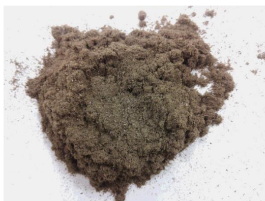
Fig. 4.31 Steam treated rice straw after milling ( \leq 1\text{mm} ).
