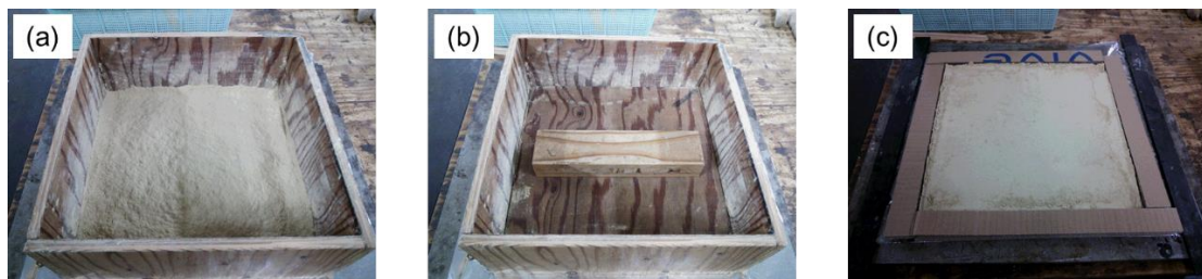
Fig.2.1 Forming procedure. (a) Raw materials inside the wood frame (Inside diameter: 30×30cm). (b) Pre-pressing. (c) Mat before pressing.
