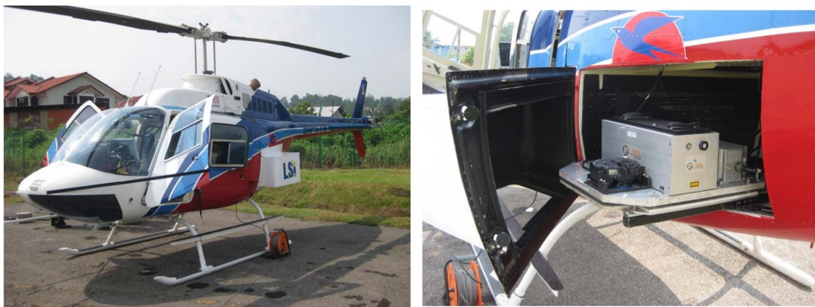
Figure 4.3: The Bell 206B3 Jet Ranger with LSI MATRIX system. The system use Riegl LMS-Q560 and Canon EOS-1D Mark III camera
