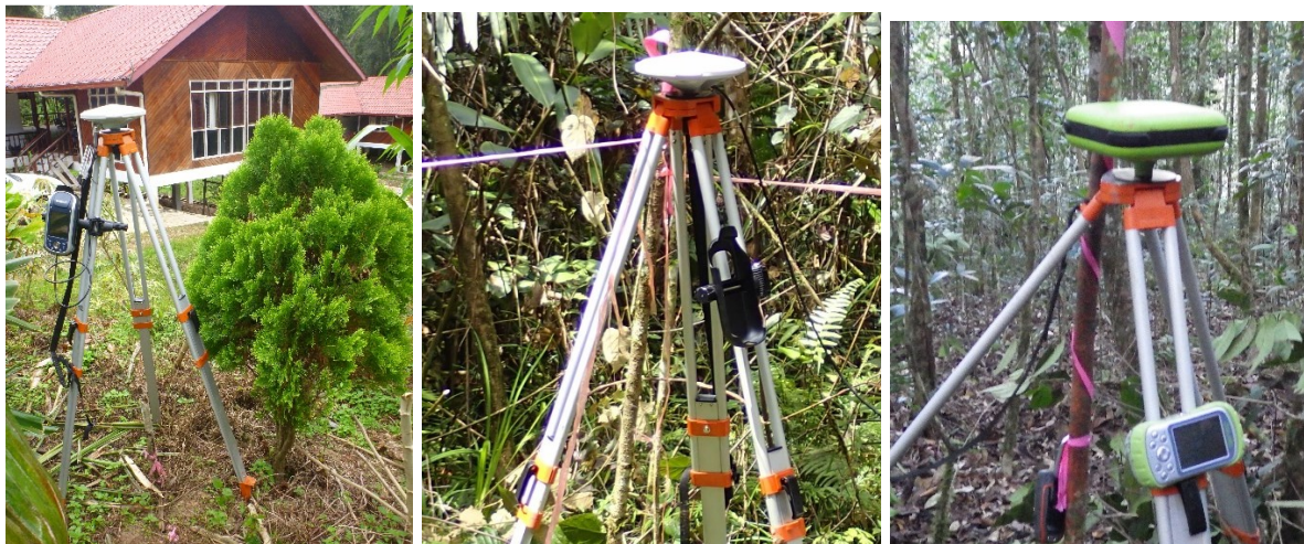
Figure 4.5:(a) GNSS base station at TBM1 (b) GNSS rover station at plot center with Ashtech Promark 100 (c) GNSS rover station at plot center with JAVAD Triumph-1.
