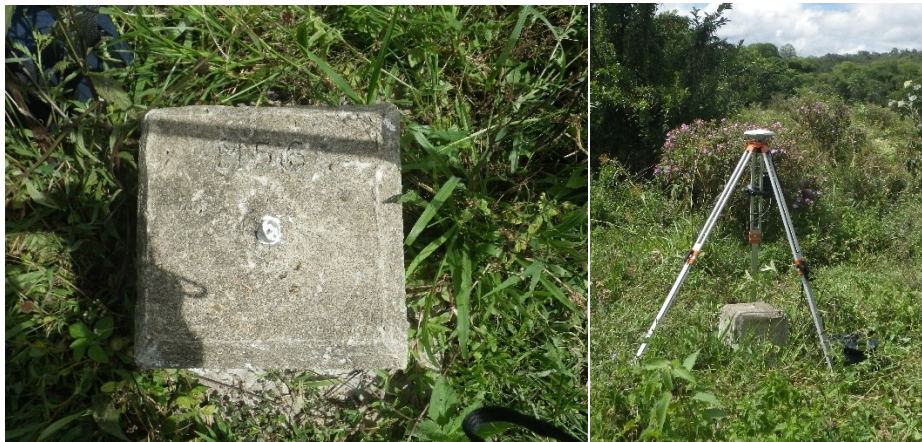
Figure 4.4: One of the base station used for control points, Base station M516 located in Kampung Long Pasia (Photo: SatAirTrop Project).
