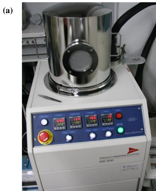
Figure 3-3 (a): Parylene coater developed by SCS company, (LABCOTER).
