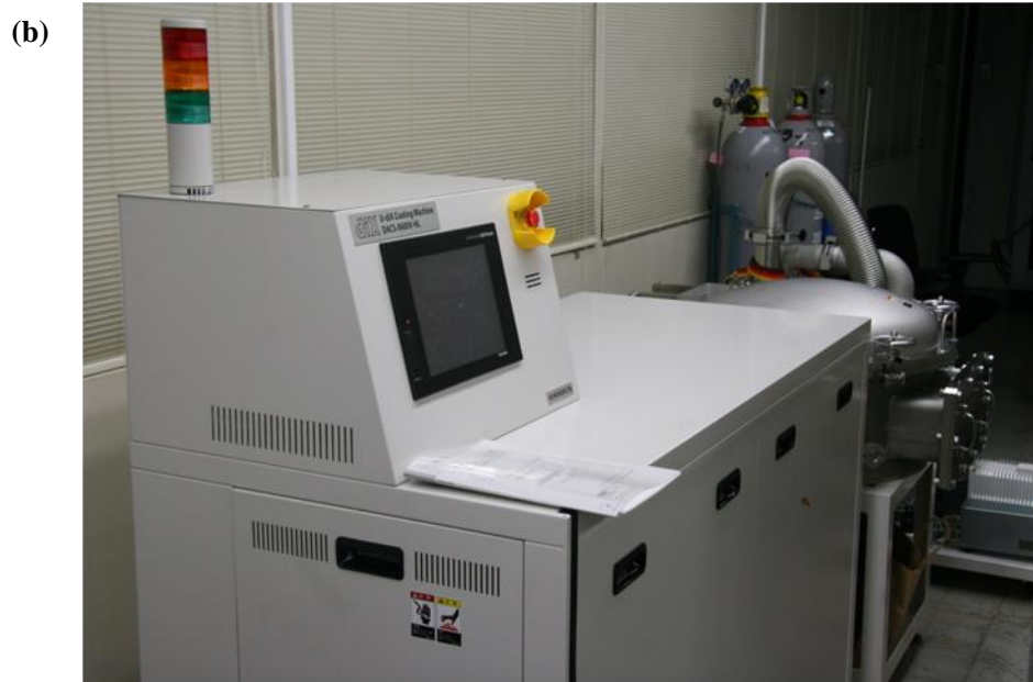
Figure 3-3 (b): Parylene coater developed by KISCO LTD., (U-diX).
