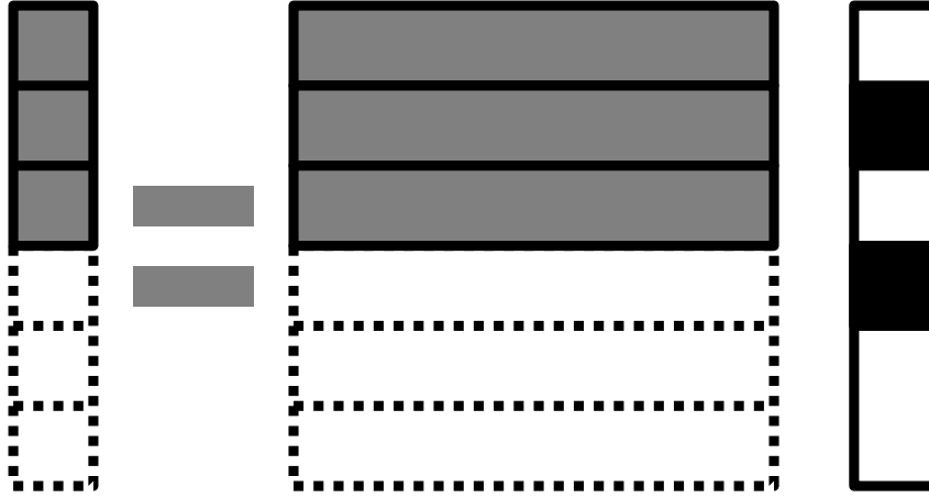
Figure 1.4: An illustration of compressed sensing, formulated by \mathbf{y} = \mathbf{A}\mathbf{x} . The case where the data \mathbf{y} is scarce, is dealt with by assuming that the original signal \mathbf{x} is sparse.
