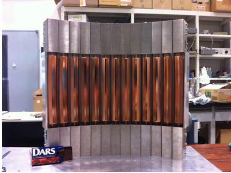
Fig. 4.1: Front view of the CCC antenna.
