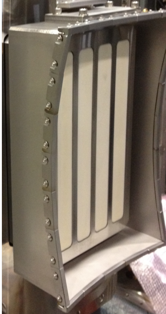
Fig. 3.9: Photograph of the grill antenna (ceramic-loaded waveguide array).
