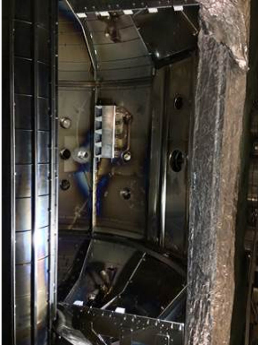
Fig. 4.11: Upper and lower z450 limiters installed at z = \pm 0.45 m. Two Langmuir probes are mounted on the upper z450 limiter. U1 probe at (R, z) = (267\text{mm}, 450\text{ mm}) and U2 probe-: at (R, z) = (464\text{mm}, 450\text{ mm}) .
