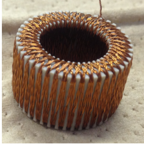
Fig. 2.5: Eight-layer Rogowski coil: Outer diameter = 20 mm; inner diameter = 12 mm; thickness = 12 mm; number of turns = 360; and cable diameter = 0.12 mm [72].
