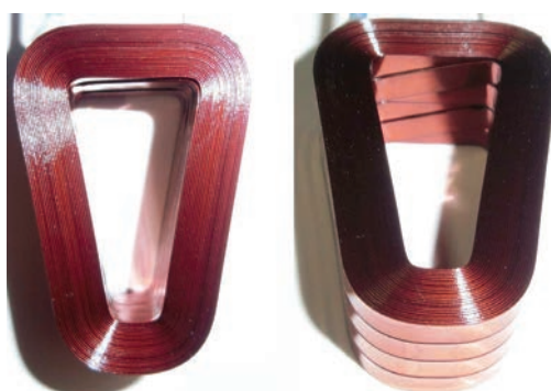
Fig. 5.4: Flat-type wire applied to the new motor
