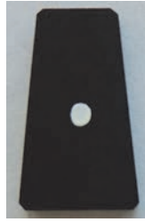
Fig. 5.4: Trapezoidal PM applied to proposed motor (ShinEtsu Rare Earth Magnets SEREM N50AS-G)
