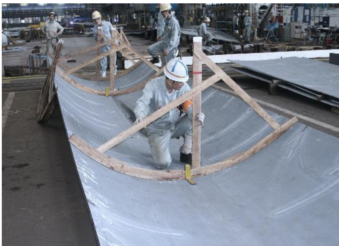
Figure 1-9 Wooden template fixing and observing
