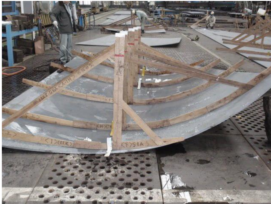
Figure 1-7 Manufacturing plan's design using wooden templates
