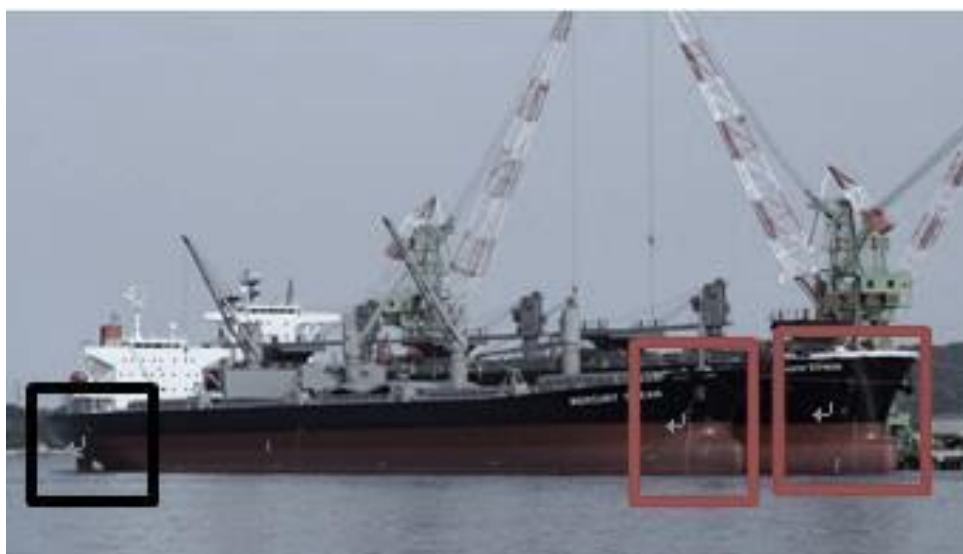
Figure 1-2 Curved shell plates on the bow and stern (Ikeda, Y. et al 2009)
