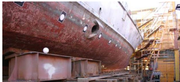
Figure 2-6 Waterline marked with black and white targets for registration of multiple laser scanners (Biskup, K. 2007)
