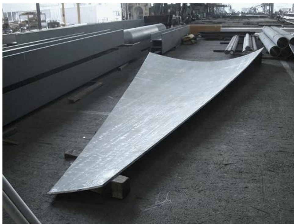
Figure 1-3 Curved shell plates on the bow and stern (Ikeda, Y. et al 2009)
