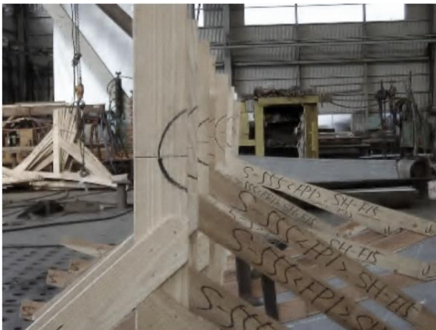
Figure 1-8 Perspective line of wooden templates
