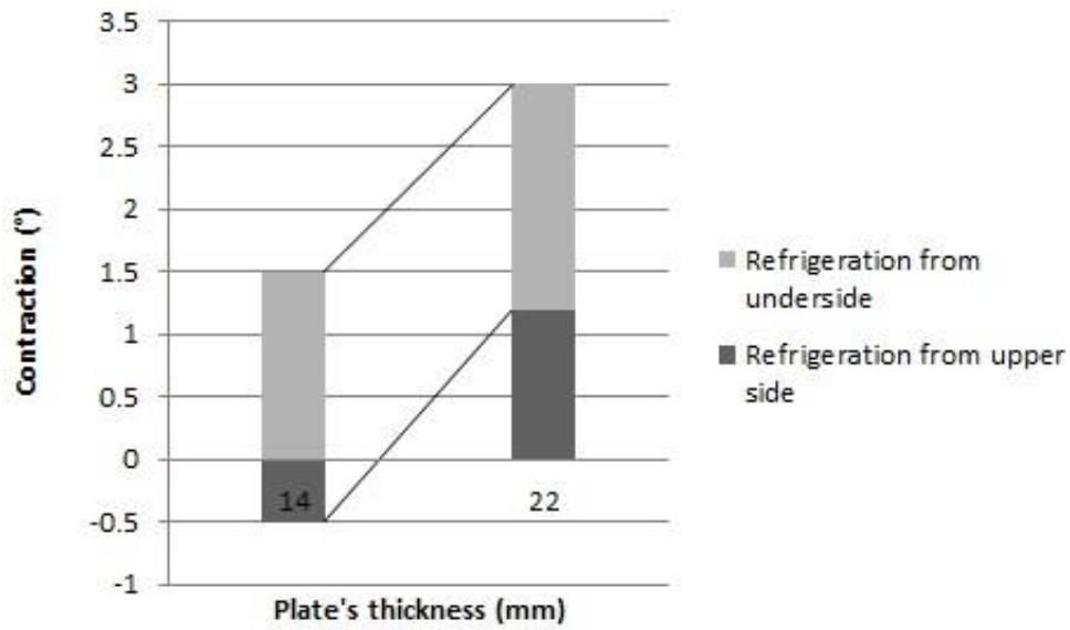
Figure a1-16 Relation between the plate's thickness and the contraction of the plate (Heating speed: 170mm/min; Heating from upper side)
