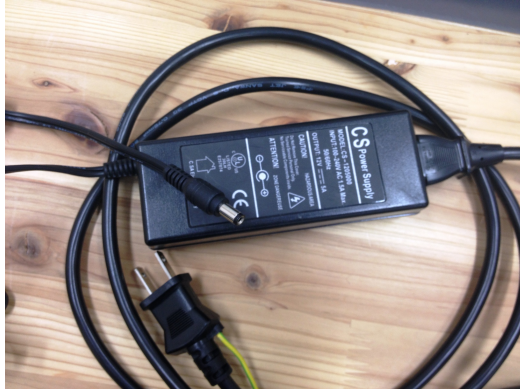
(a) Power supply: 100VAC 50/60Hz input, 12VDC output.
