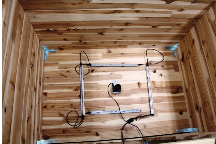
Figure 3.7: Inside view of the tabletop interface. The camera is positioned on the center of the bottom of the box and it is surrounded by infrared LED tubes.
