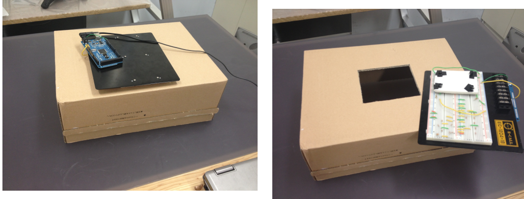
(a) Box and breadboard with the marker attached on it during an experiment for height h = 10\text{cm} .
