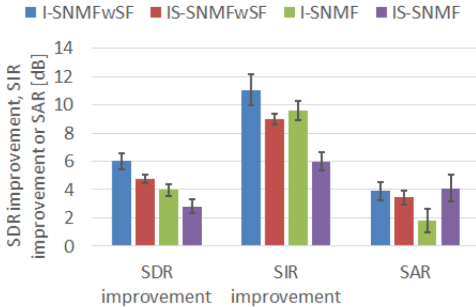
Figure 3.2: Average SDR improvements, SIR improvements and SARs with standard errors for overall data. The parameters and algorithms are the same as Table 3.2.
