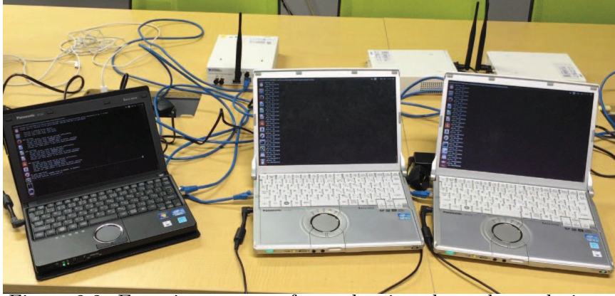
Figure 2.2: Experiment setup for evaluating channel correlations.
