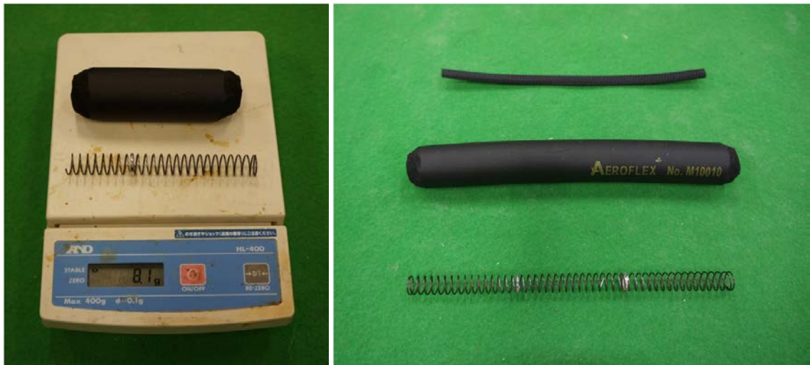
図 6.26: Muscle wire cover newly proposed for Kengoro.[89]
