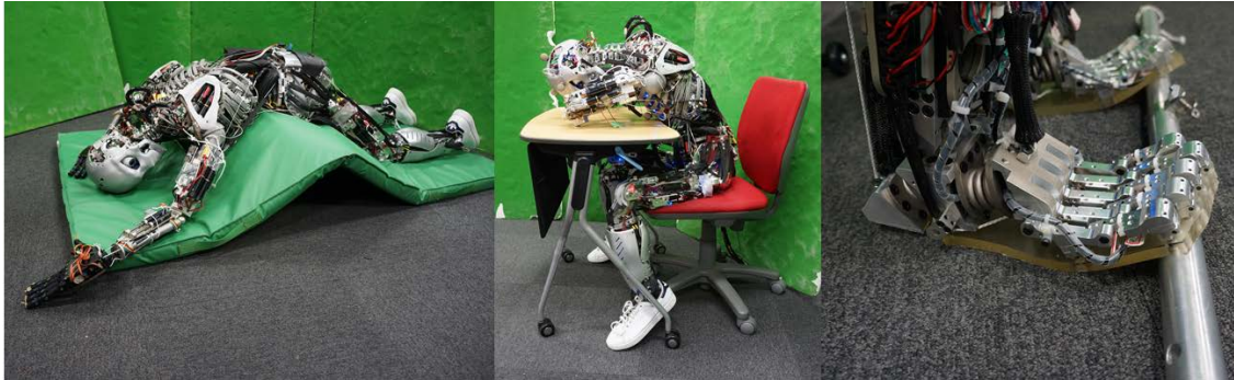
図 2.6: Adapting to the environment by using musculoskeletal flexible joint structures.
