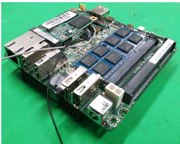
図 6.18: Small brain PC(intel NUC) inside Kenshiro head.
