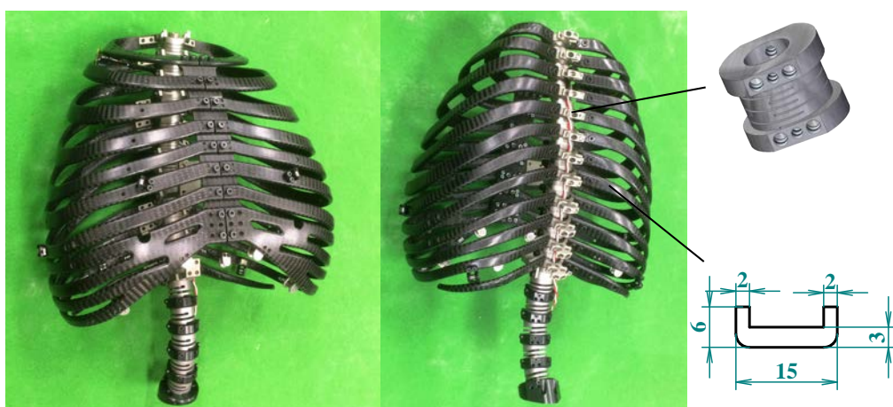
図 6.29: Overview of the rib cage, thoracic and lumber vertebrae. Rib cage is made from CFRP. The rib cage was designed to keep its flexibility to keep the DOF in the thoracic vertebrae. 12 cervical vertebrae and 5 lumber vertebrae can be seen. [89]
