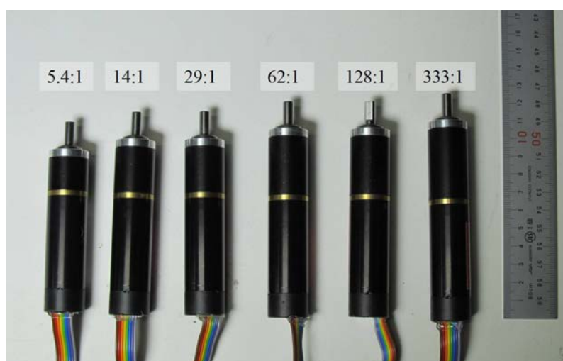
図 6.4: From 0 to 65mm is motor part. Head part than 65mm is gear. From the right, 5.4:1(1stage 39mm) / 14:1,29:1(2stages 45mm) / 62:1,128:1(3stages 52mm) / 333:1(4stages 59mm) [75].
