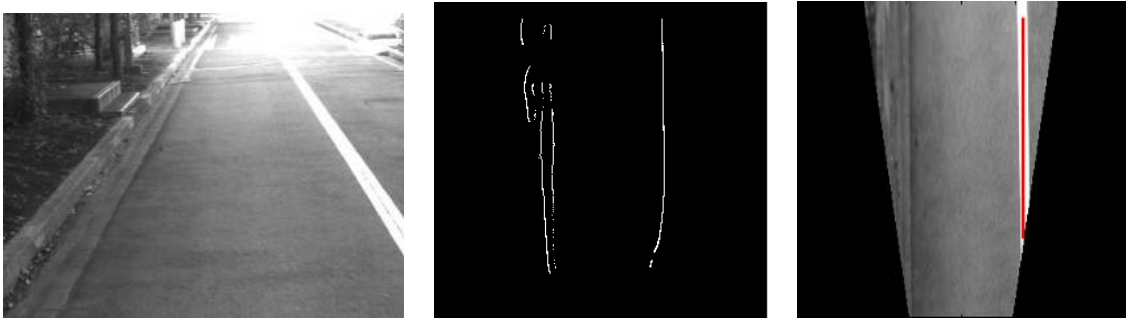
Fig.B. 5 Image processing results (from left to right: original image, Binarized image, Lane fitting result).
