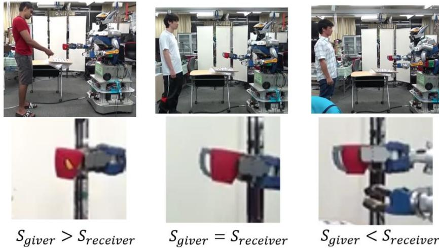
**Figure 6-16 Handover execution. In each case, HRP2V handed over the mug using an appropriate grasp configuration matching the demonstrated one.**
