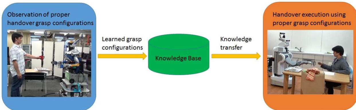
**Figure 6-20 Knowledge transfer between robots. The handover grasp configurations learned by HRP2V are stored into a knowledge base. This knowledge is then transferred to PR2. PR2 then utilizes this transferred knowledge to execute handovers properly.**
