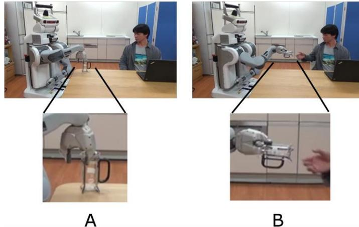
**Figure 6-18 Improper handover of a mug. A – Robot inserts finger into mug. B – Robot hands over mug sideways.**
