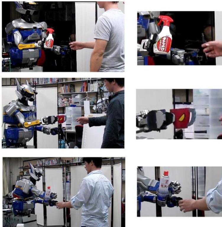
**Figure 6-9 Handover execution in the first set of experiments using learned grasp configurations. The robot successfully handed over all three objects using grasp configurations that match the ones demonstrated to it by the person previously. (Published in Chan et al. 2015 [131].)**
