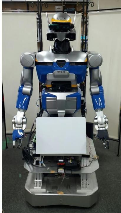
**Figure 6-4 Kawada Industries HRP2V Robot with ASUS Xtion Pro Live camera mounted on the head. (Published in Chan et al. 2015 [131].)**
