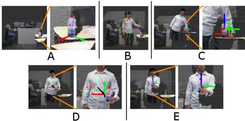
Figure 6-5 Stages of extracting grasp configurations from handover demonstrations. A – Object detection. B – Human detection and tracking. C – Grasp point detection. D – Direction of torso-to-hand vector for handover cue detection. E – Object orientation at handover. (Published in Chan et al. 2015 [131].)
