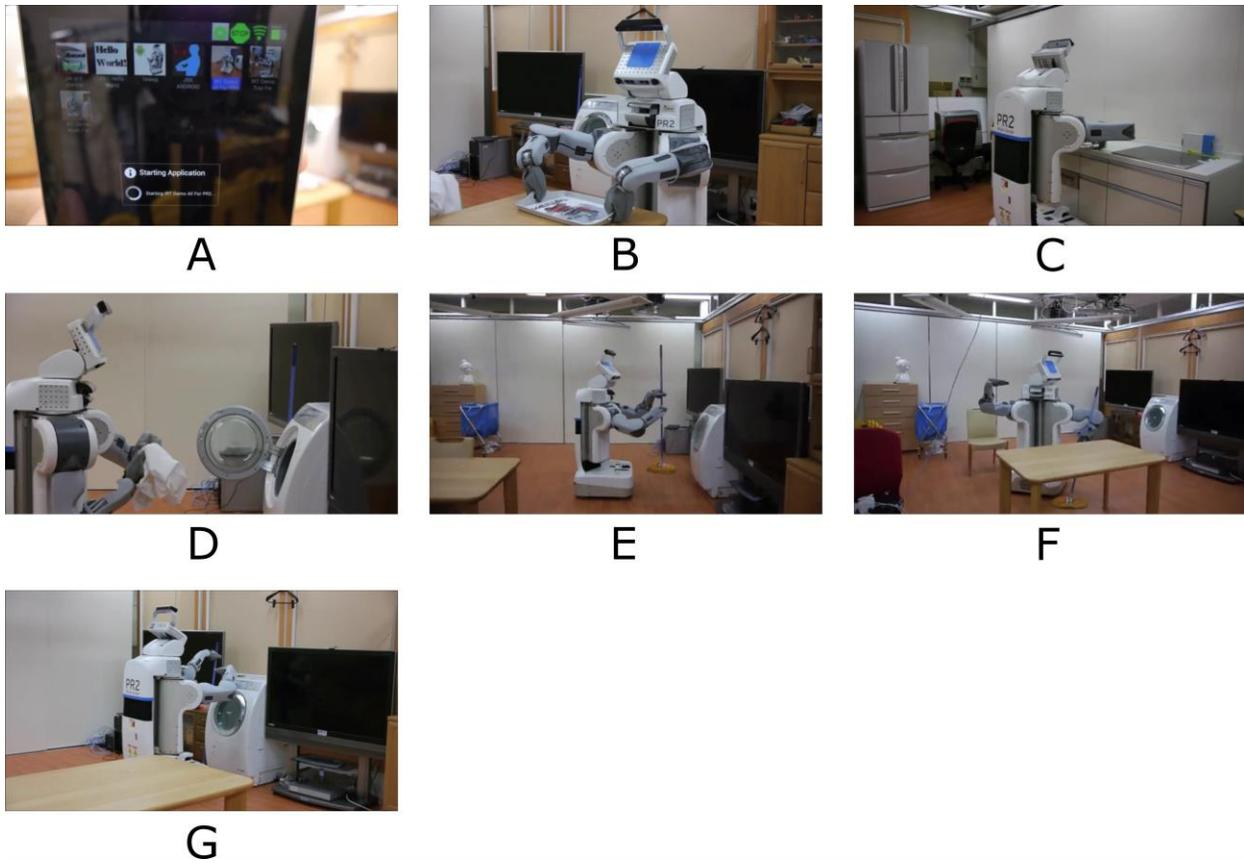
**Figure 6-17 A household robot performs cleaning tasks. The users sends the command through a tablet device (A). The robot picks up an empty tray from the table (B), and brings the tray to the kitchen counter (C). Robot puts clothes into the washing machine (D), picks up the broom (E), sweeps underneath the table (F), and places broom back (G).**
