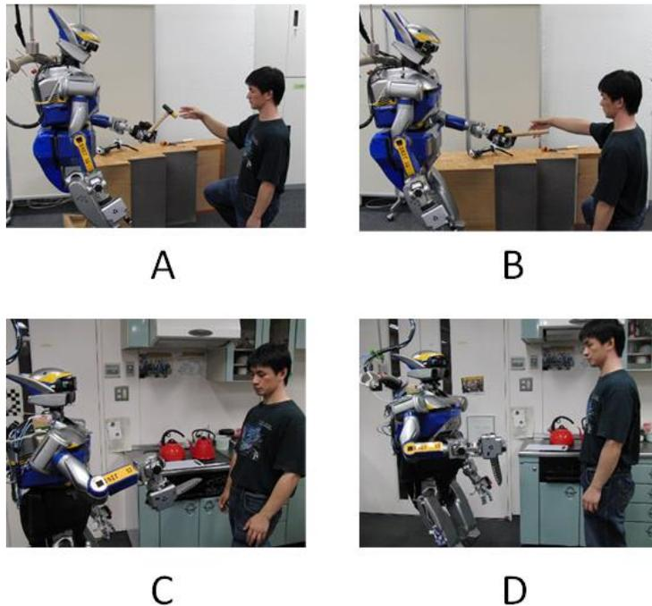
**Figure 1-1 Comparison of handover grasp configurations for hammer and kitchen knife. (Published in Chan et al. 2013 [44].)**
