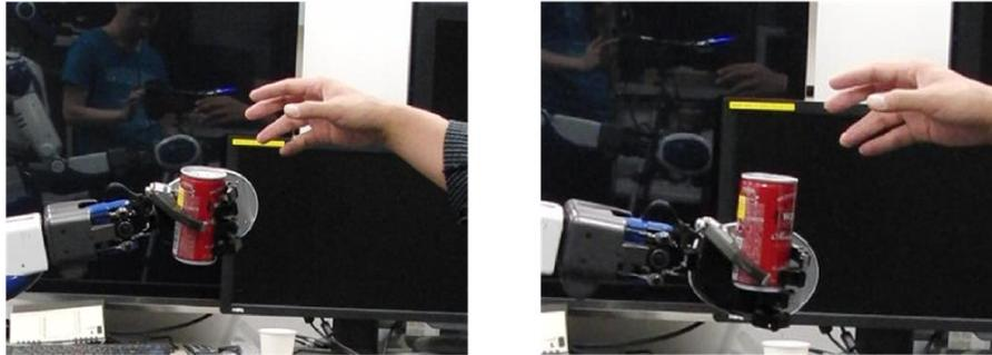
**Figure 2-1 Comparison of handover grasp configurations for a can of coffee. (Published in Chan et al. 2013 [38].)**
