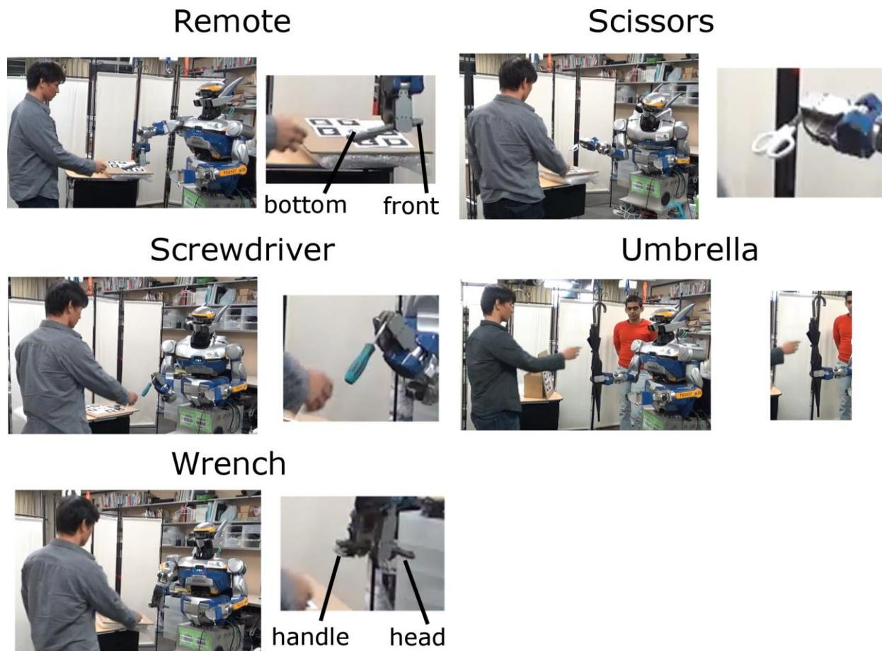
**Figure 6-11 Handover execution using learned grasp configurations during qualitative evaluation in the second set of experiments. Figure shows the grasp configurations used for the last five objects of the fifteen objects used in the second set of experiments.**
