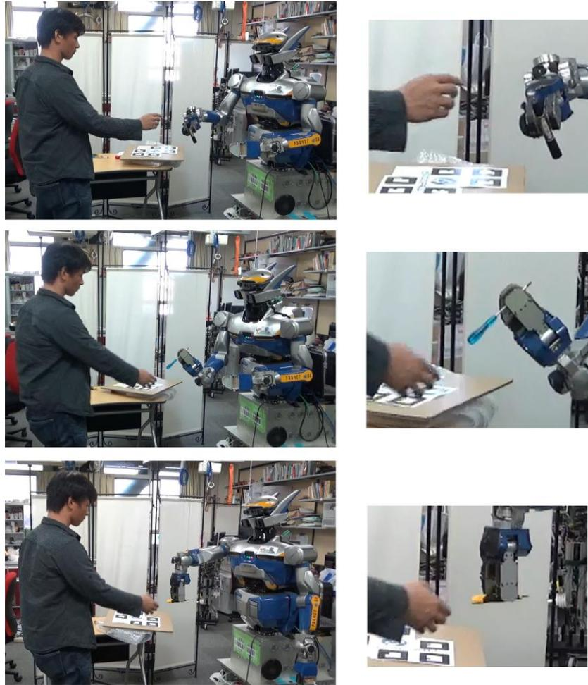
**Figure 6-12 Handover execution of new objects, showing grasp configuration used for the marker pen, screwdriver, and cutter from top to bottom.**
