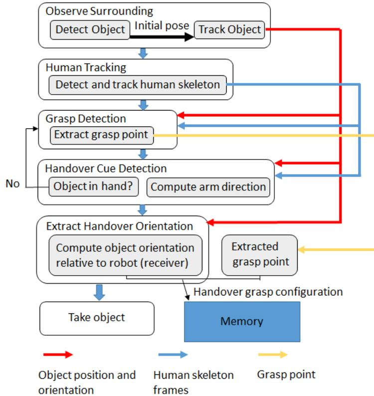
**Figure 6-1 Flow diagram of system for extracting handover grasp configurations from handovers with users.**
