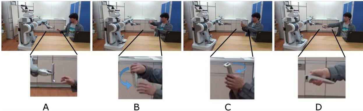
**Figure 6-19 Improper handover of a remote. A – robot hands over remote upside down with buttons facing away from user. B – After taking the remote, the user needs to first turn the remote upright. C – User then needs the turn the remote around to see the buttons. D – Finally, user can use the remote.**
