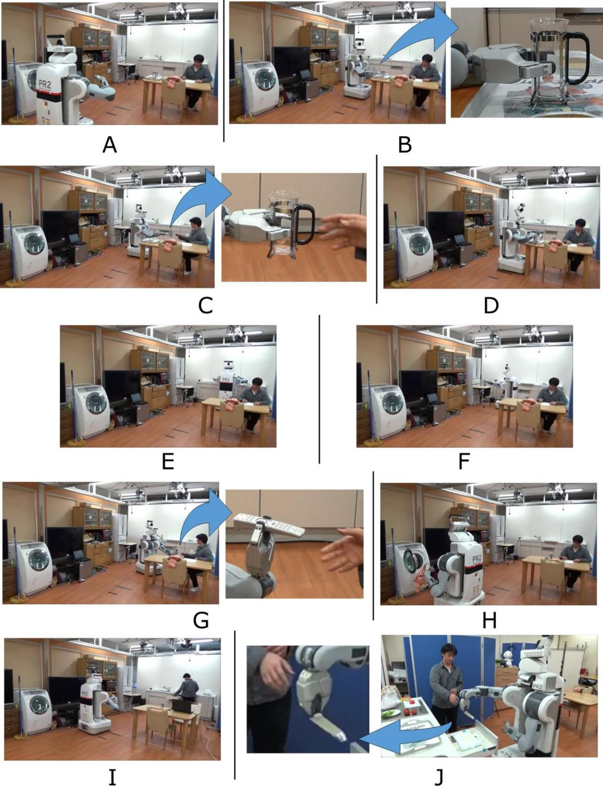
Figure 6-21 integration experiment. A – PR2 in room with person. B – Pick up mug. C – Hand over mug. D – Pick up tray. E – Place tray at counter. F – Pick up remote. G – Hand over remote. H – Place clothes in washing Machine. I – Move to kitchen. J – Hand over kitchen knife.
