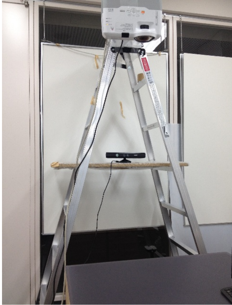
Figure 4.2: System configuration: the Kinect acquires the user's current head and hand position and two projectors are used, for the paper projection and the tabletop projection
