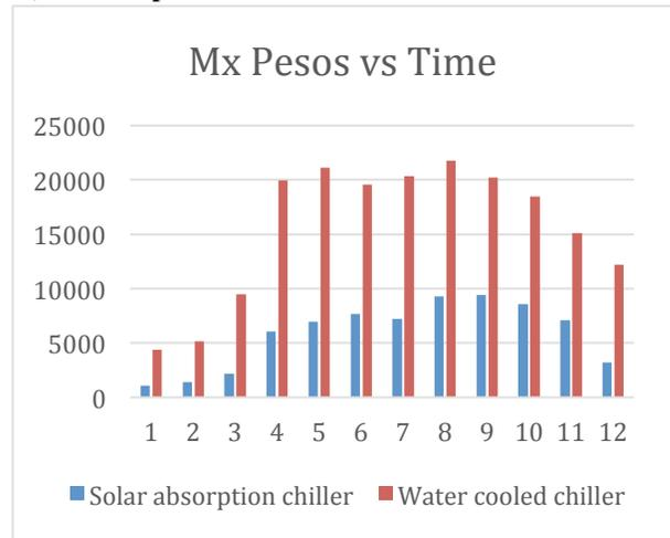
**Figure 4.** Annual cost comparison between the solar absorption chiller and a traditional water-cooled chiller.
