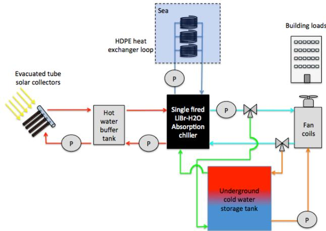
**Figure 1.** Diagram of the design of the proposed solar absorption chiller system
