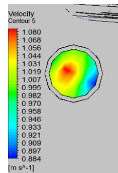
Figure 2. Velocity contour at the outlet of the helical coil
