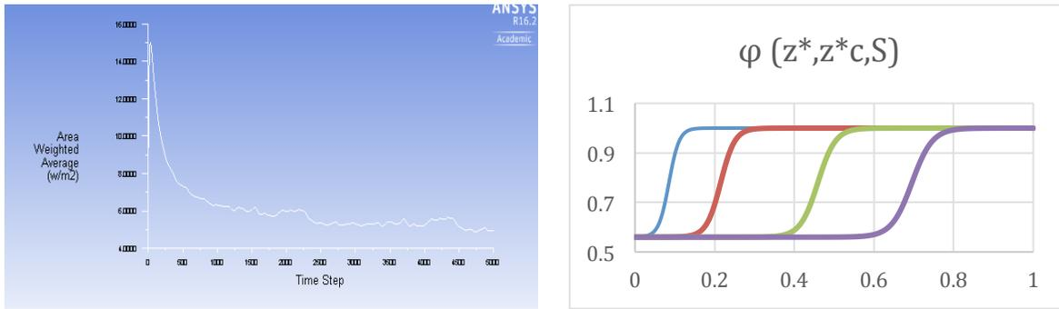
**Figure 3.** a) Change in area weighted heat flux as a function of time in the underground thermal storage tank, b) dimensionless thermocline temperature in function of the dimensionless height during charge.
