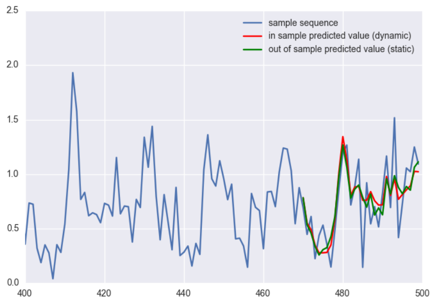
FIGURE 3.6: The comparison of two prediction types. In this figure, the data size for in-sample prediction is 500 with the prediction size 30, while the data size for out-of sample prediction is 470.
