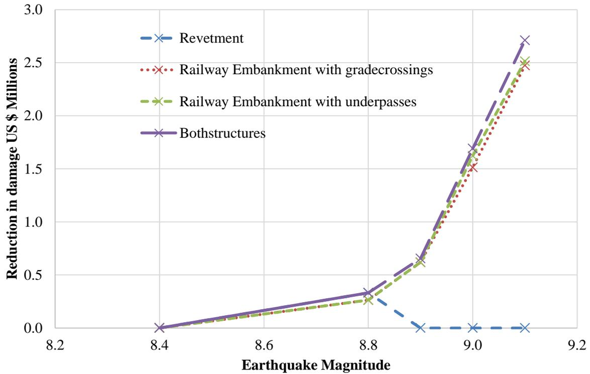
Figure 95: Reduction in damage vs. earthquake magnitudes (for the case when the tsunami co-beneficial structures collapse due to tsunami overflow) (Schematic diagram)
