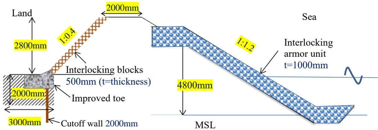
Figure 77: Schematic diagram of proposed modifications to the revetment (cross section)
