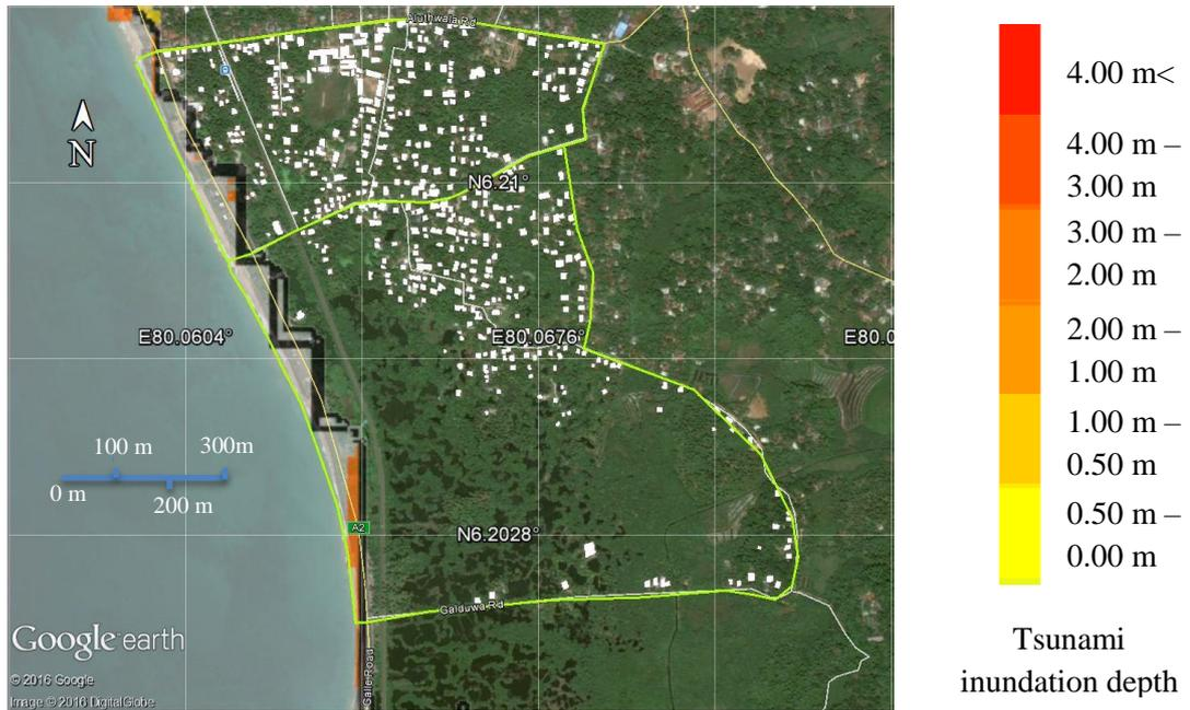
Figure 25: Tsunami inundation depth – Scenario 1 (Mw = 8.4)
