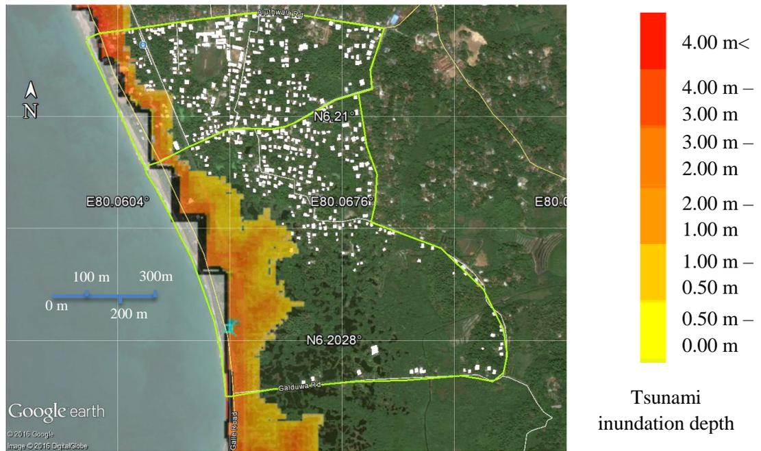
Figure 44 – Tsunami inundation depth – Scenario7 (Mw = 9.0)
