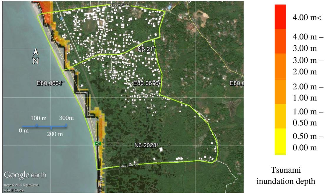
Figure 49: Tsunami inundation depth – Scenario 7 (Mw = 8.9)
