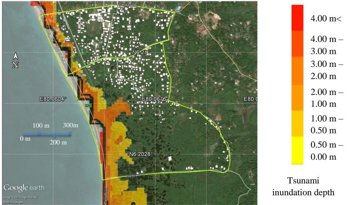
Figure 27: Tsunami inundation depth – Scenario 2 (Mw = 8.9)
