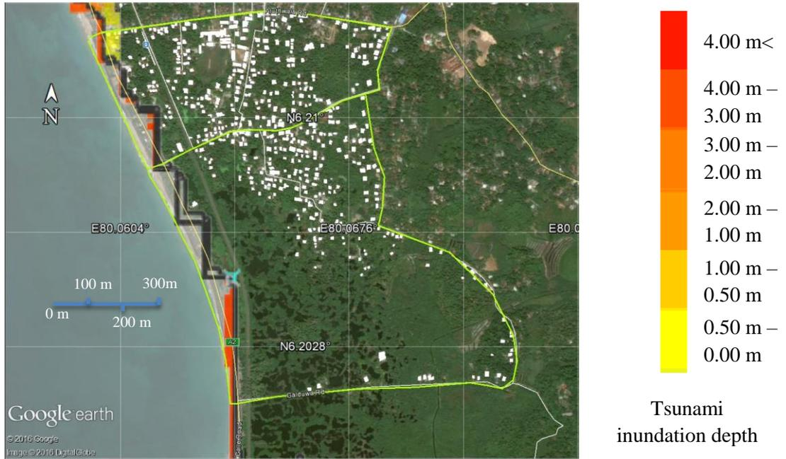
Figure 26: Tsunami inundation depth – Scenario 2 (Mw = 8.8)
