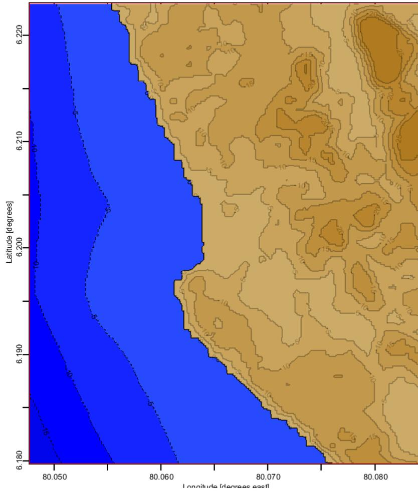
Figure 110: DEM (0.166 arcsecond resolution) (Opened using ComMIT) Contour interval: 5m)
