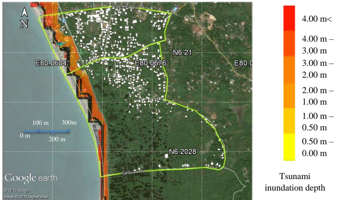
Figure 41: Tsunami inundation depth – Scenario 5 (Mw = 9.0)
