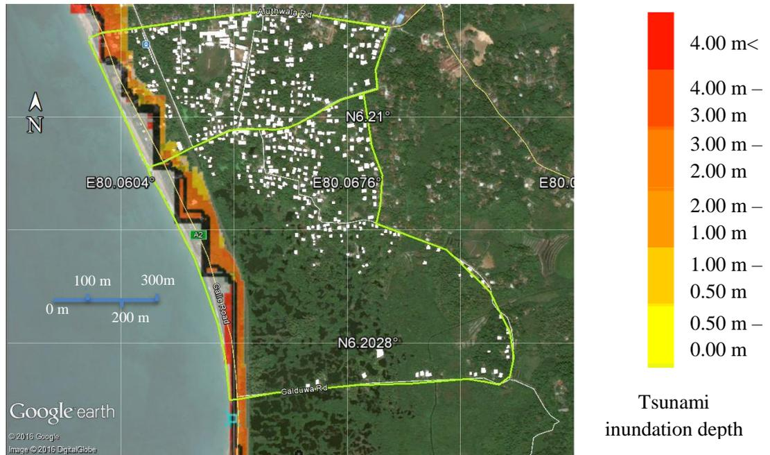
Figure 40: Tsunami inundation depth – Scenario 5 (Mw = 8.9)
