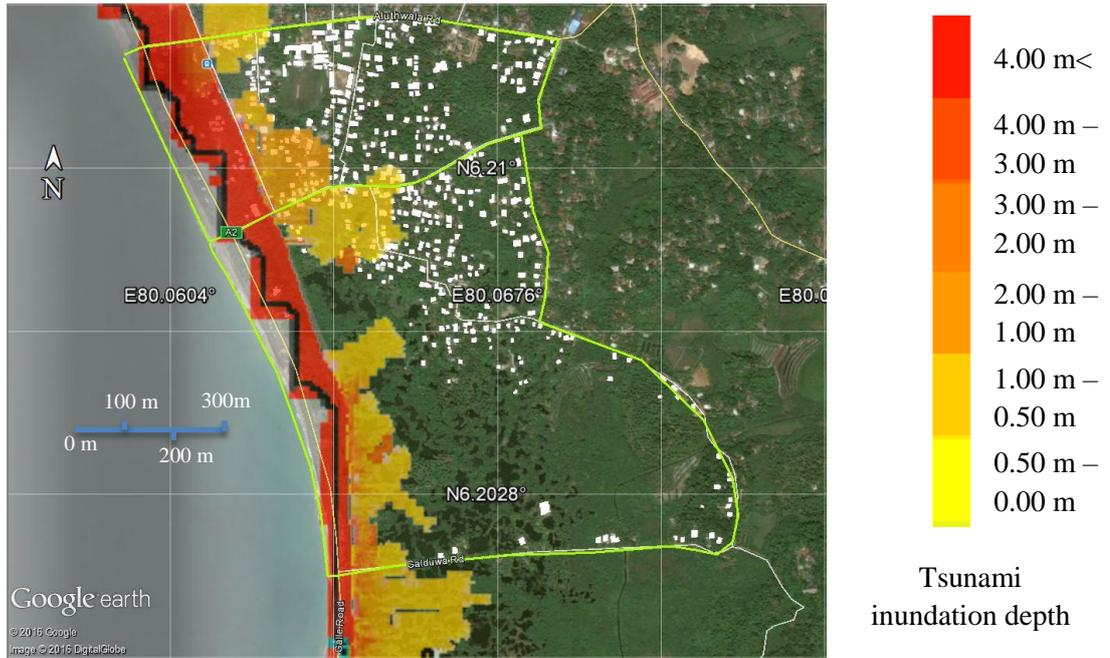
Figure 39: Tsunami inundation depth – Scenario 4 (Mw = 9.1)
