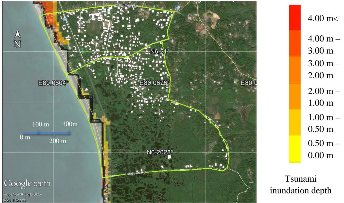
Figure 50: Tsunami inundation depth – Scenario 8 (Mw = 8.9)
