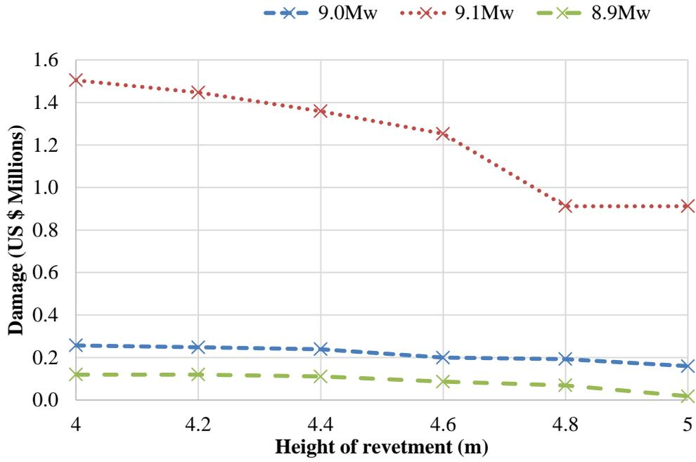
Figure 99: Damage vs. height of revetment
