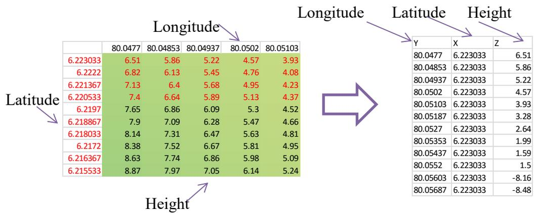
Figure 106: DEM in column format (Right hand side) and matrix format (Left hand side)
