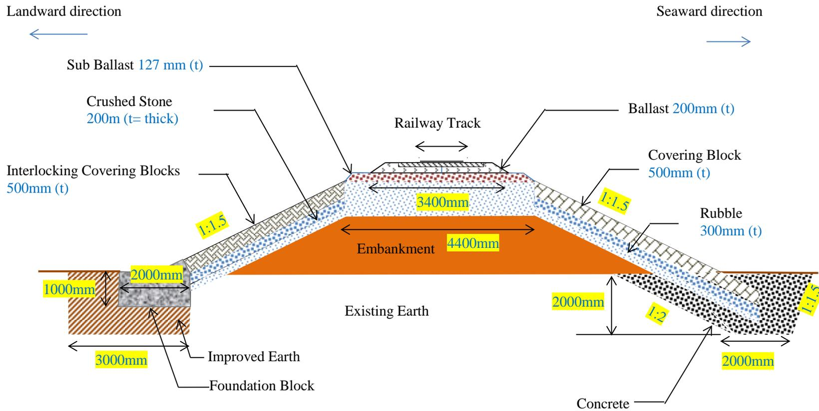
Figure 74: Schematic diagram of proposed modifications to railway embankment
