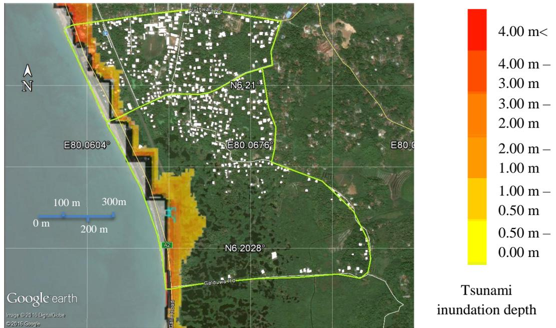
Figure 48: Tsunami inundation depth – Scenario 6 (Mw = 8.9)
