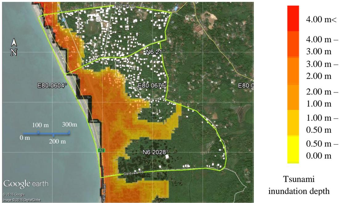
Figure 43: Tsunami inundation depth – Scenario 6 (Mw = 9.0)
