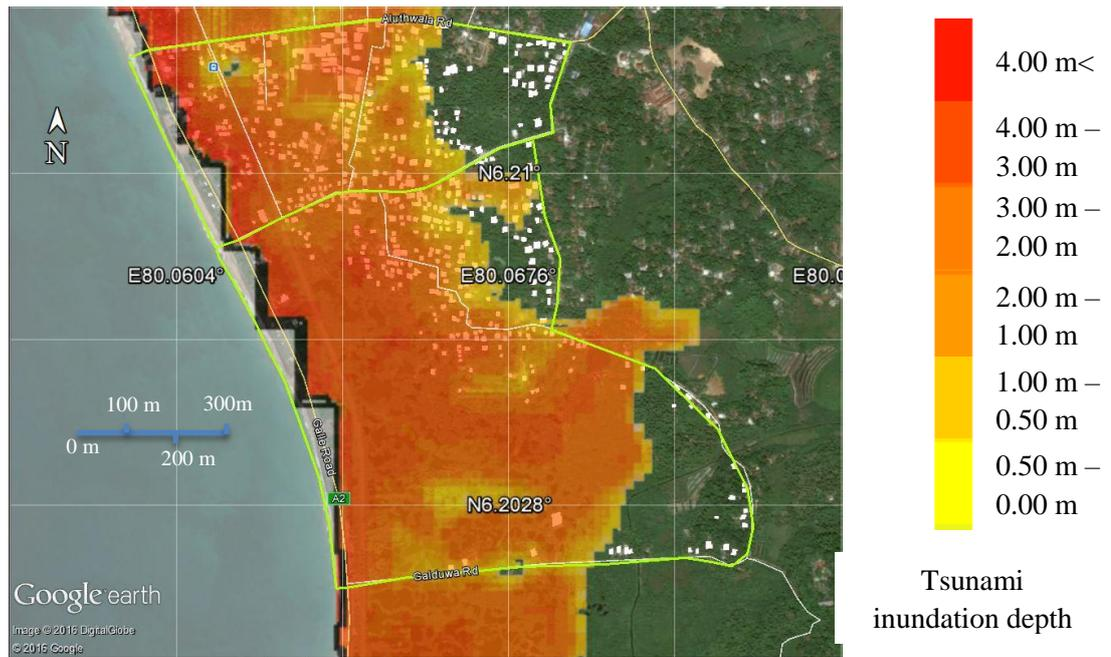
Figure 55: Tsunami inundation depth – Scenario 8 (Mw = 9.0)
