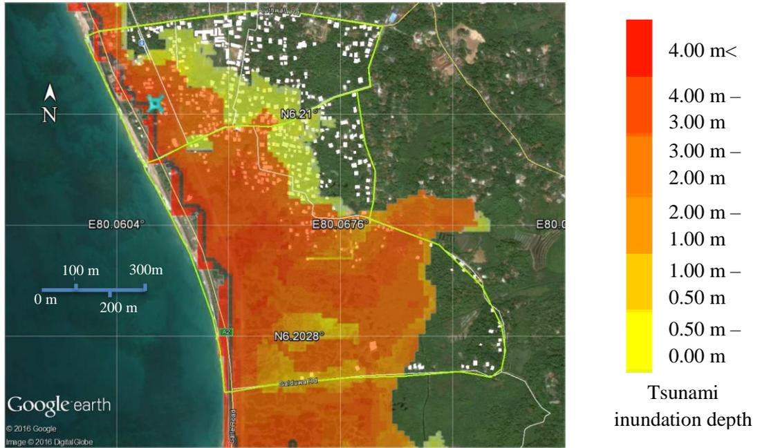
Figure 22: Tsunami inundation depth – Scenario 1 (Mw = 8.9)
