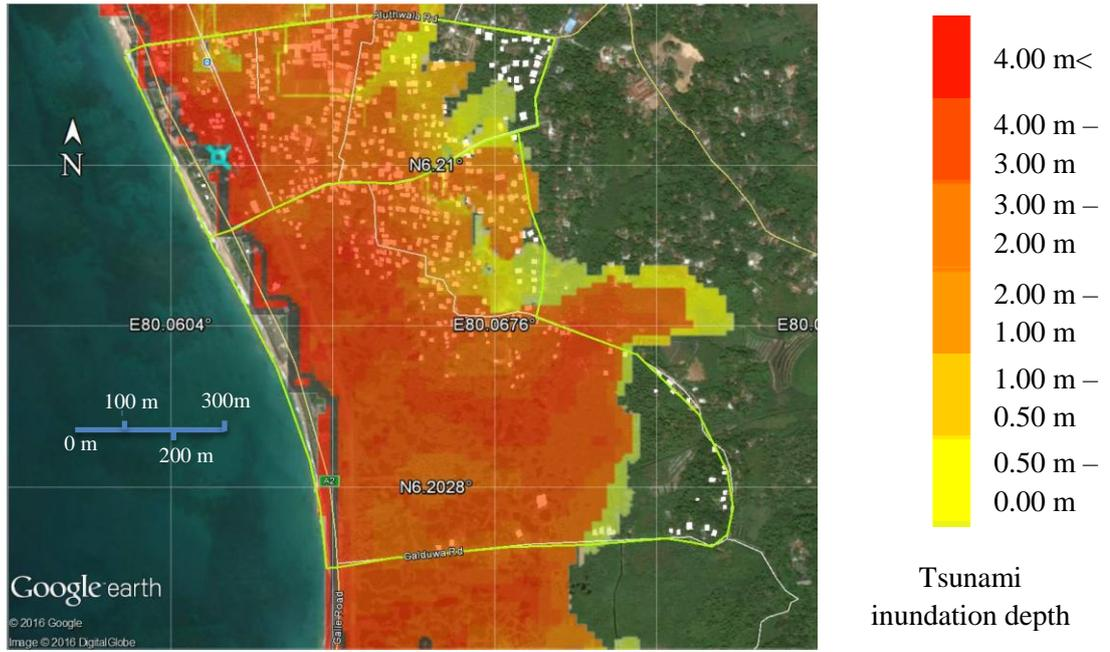
Figure 29: Tsunami inundation depth – Scenario 2 (Mw = 9.1)
