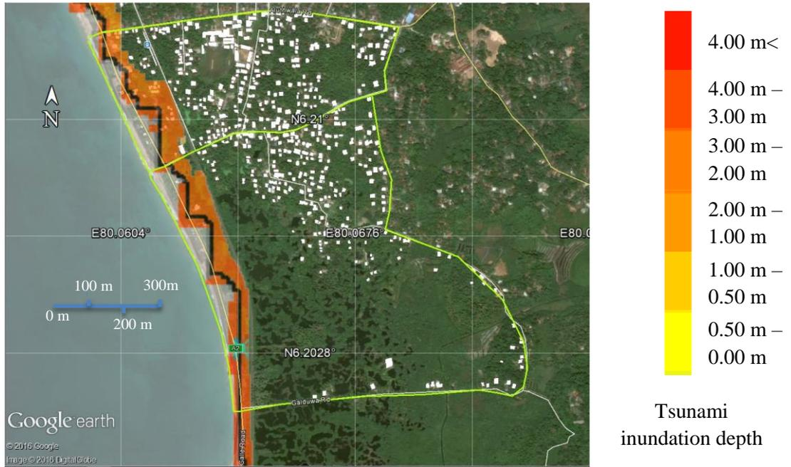
Figure 37: Tsunami inundation depth – Scenario 4 (Mw = 8.9)
