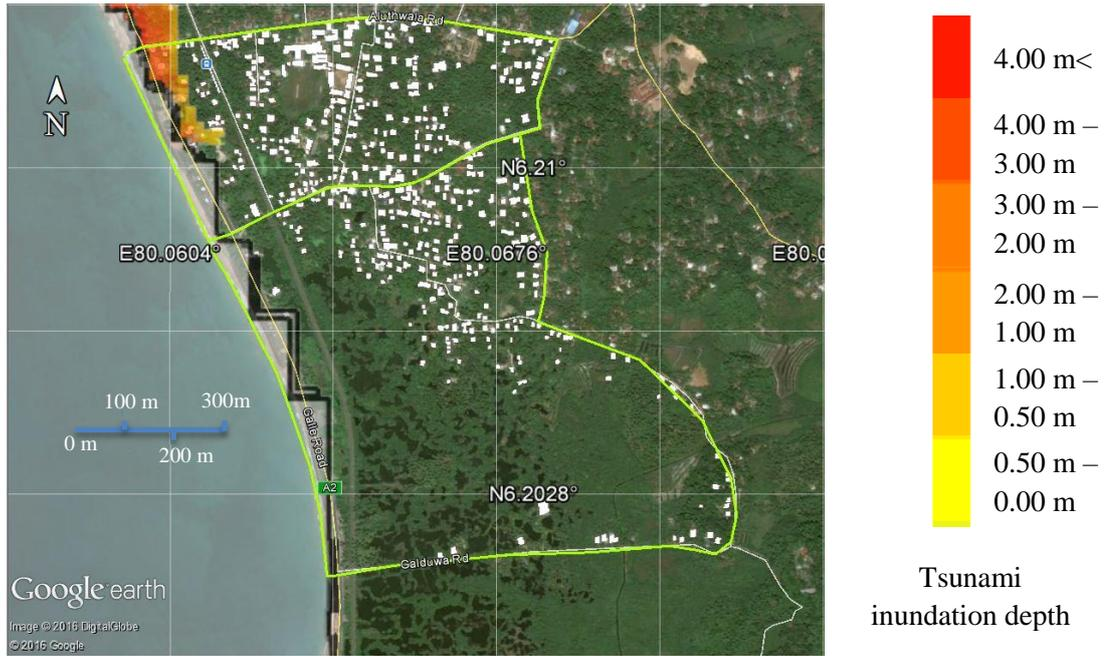
Figure 51: Tsunami inundation depth – Scenario 9 (Mw = 8.9)
