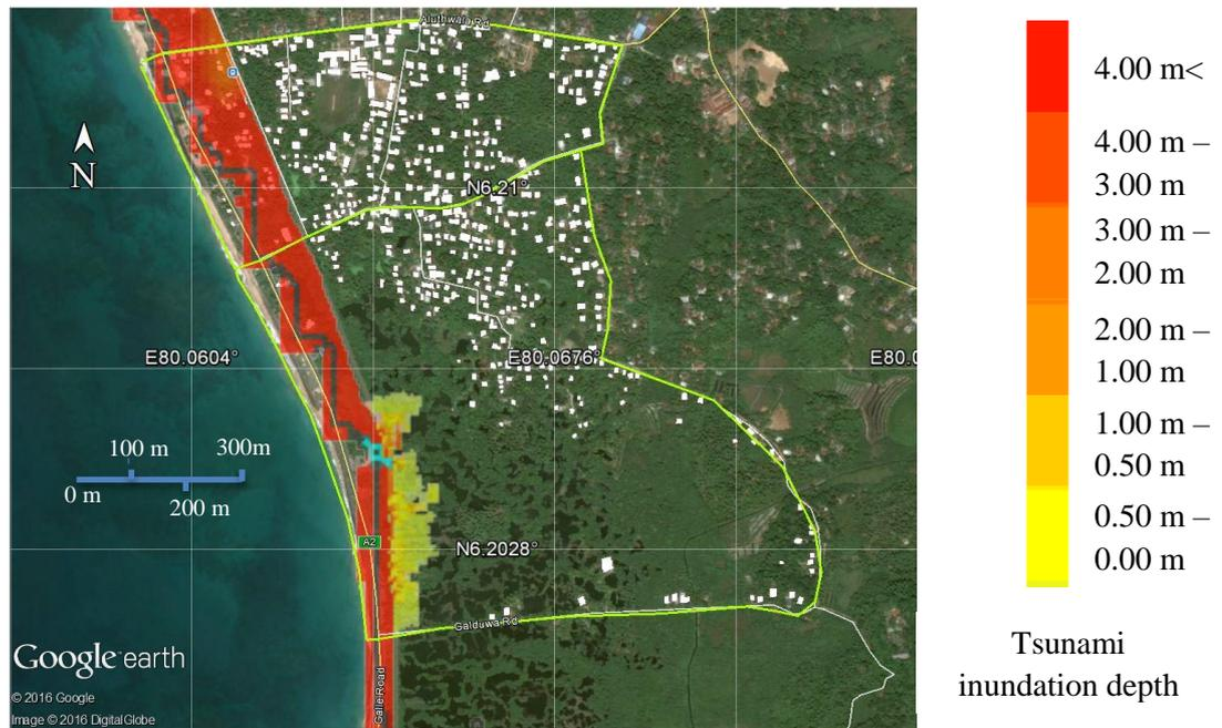
Figure 42: Tsunami inundation depth – Scenario 5 (Mw = 9.1)
