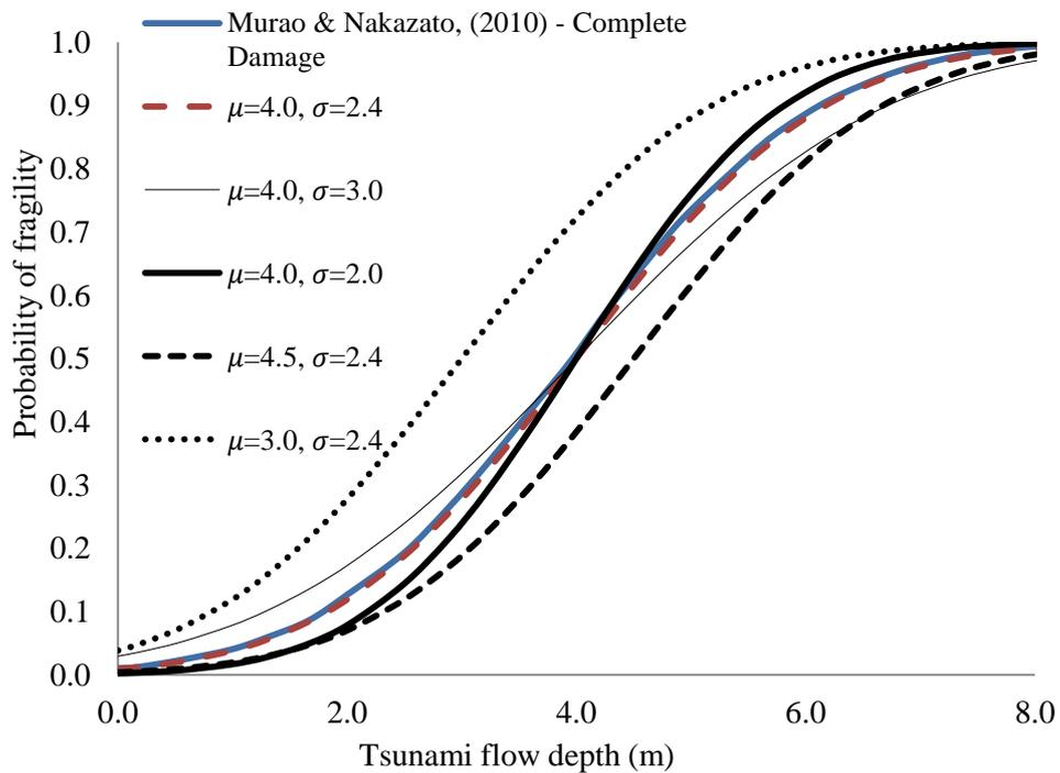
Figure 59: Fragility function of  $\Phi \left\{ \frac{H-\mu}{\sigma} \right\}$  – Different trials in iteration process
