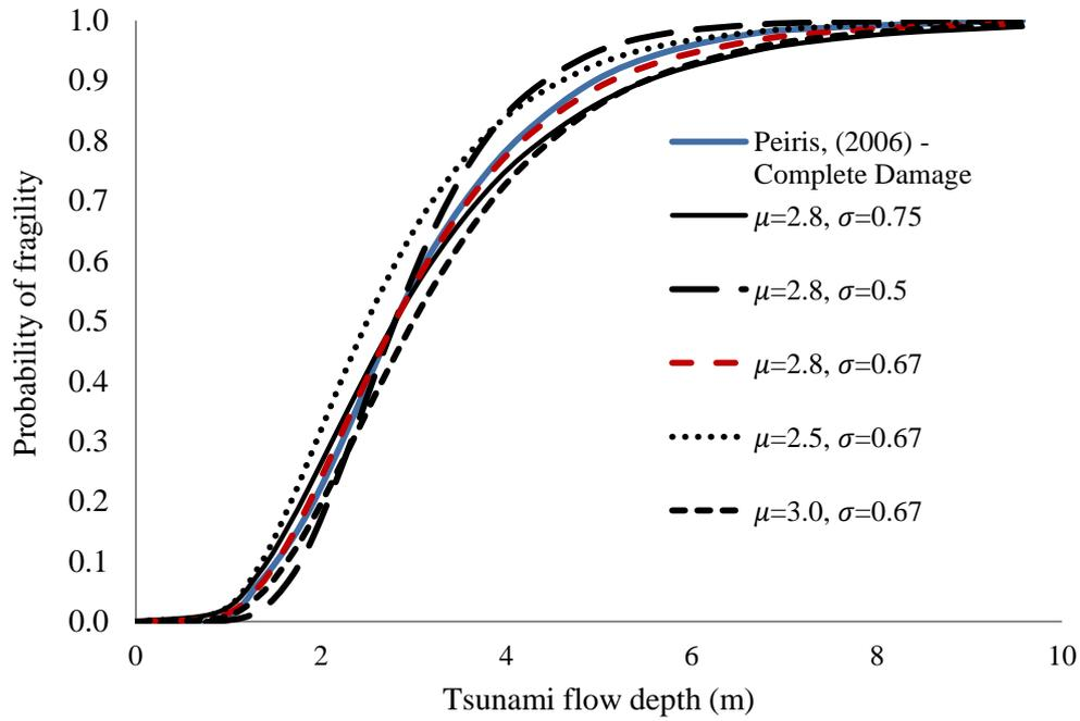
Figure 60: Fragility function of  $\Phi \left\{ \frac{1}{\sigma} \ln \left( \frac{H}{H_0} \right) \right\}$  – Different trials in iteration process
