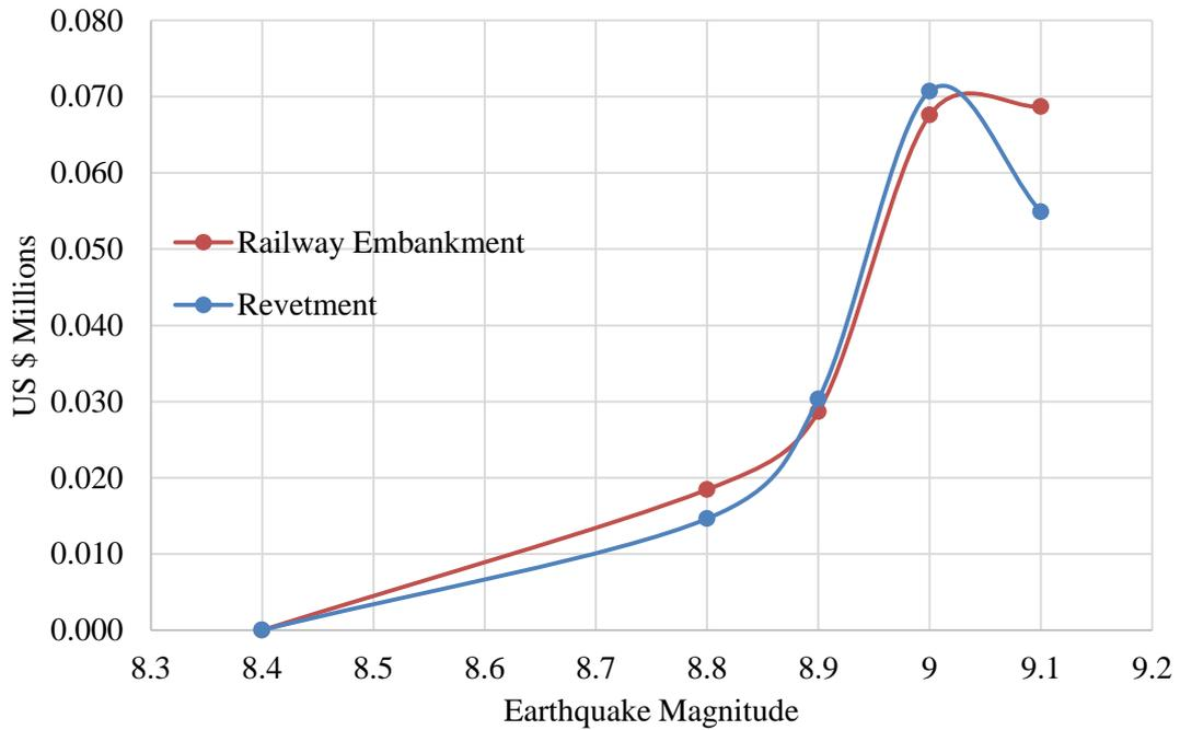
Figure 80: Expected reduction in damage of railway embankment and revetment
