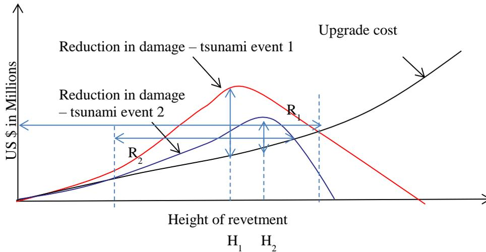
Figure 101: Expected reduction in damage and upgrading cost vs. height of the revetment (Schematic diagram)
