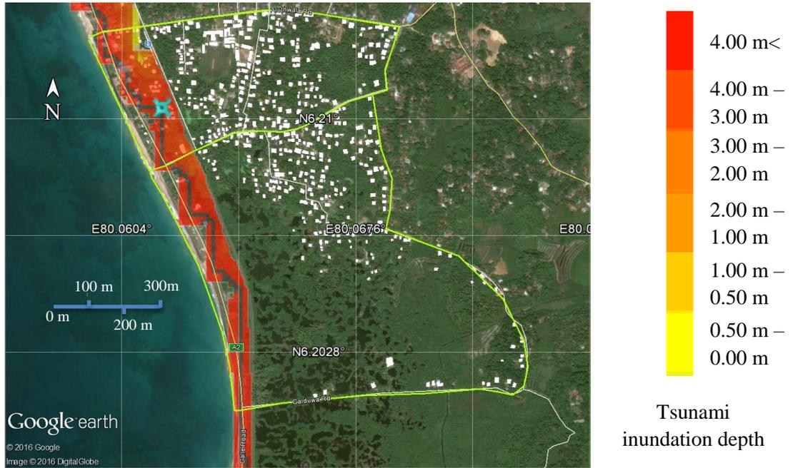
Figure 33: Tsunami inundation depth – Scenario 3 (Mw = 9.0)
