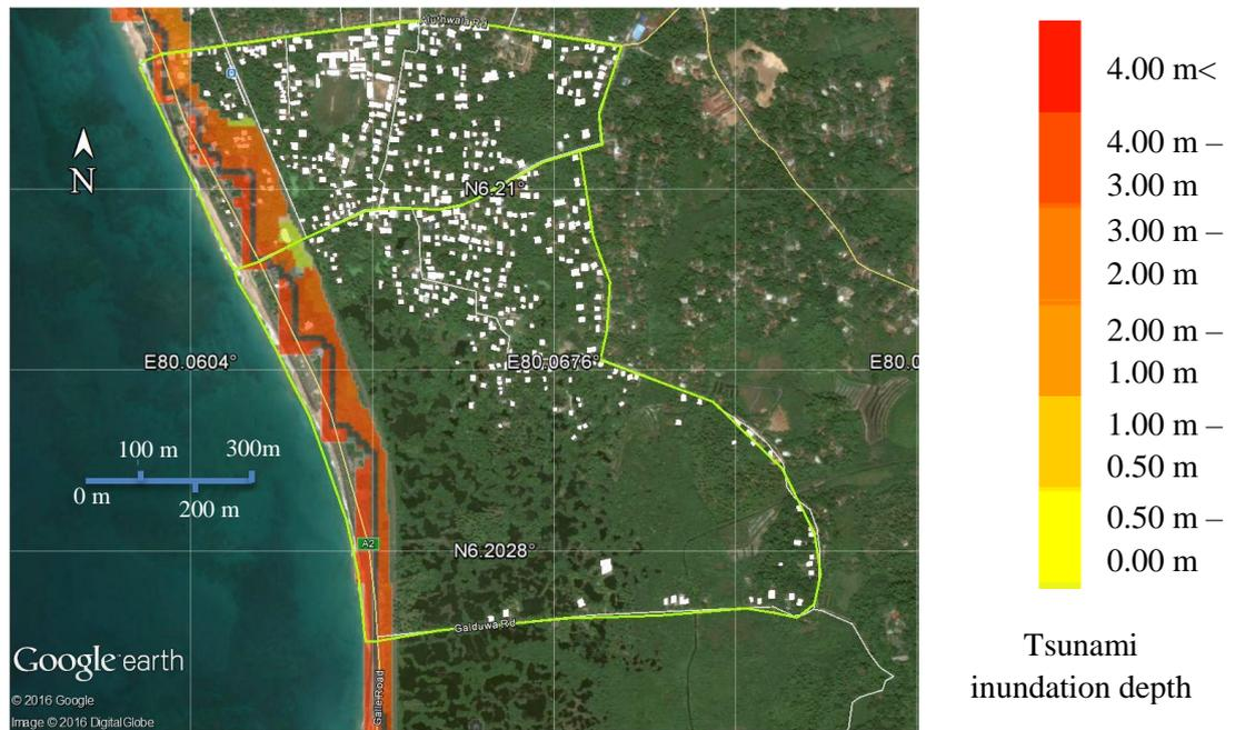
Figure 31: Tsunami inundation depth – Scenario 3 (Mw = 8.8)
