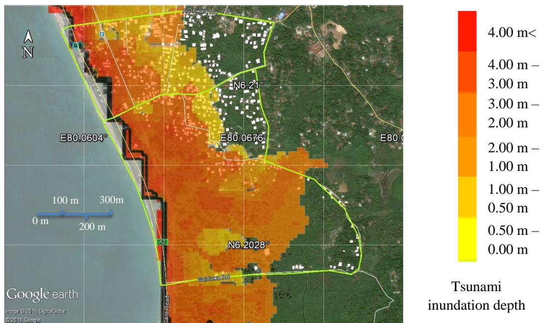
Figure 57: Tsunami inundation depth – Scenario 10 (Mw = 9.0)
