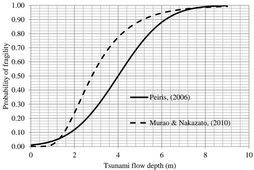
Figure 61: Comparison of selected tsunami fragility function in Sri Lanka
