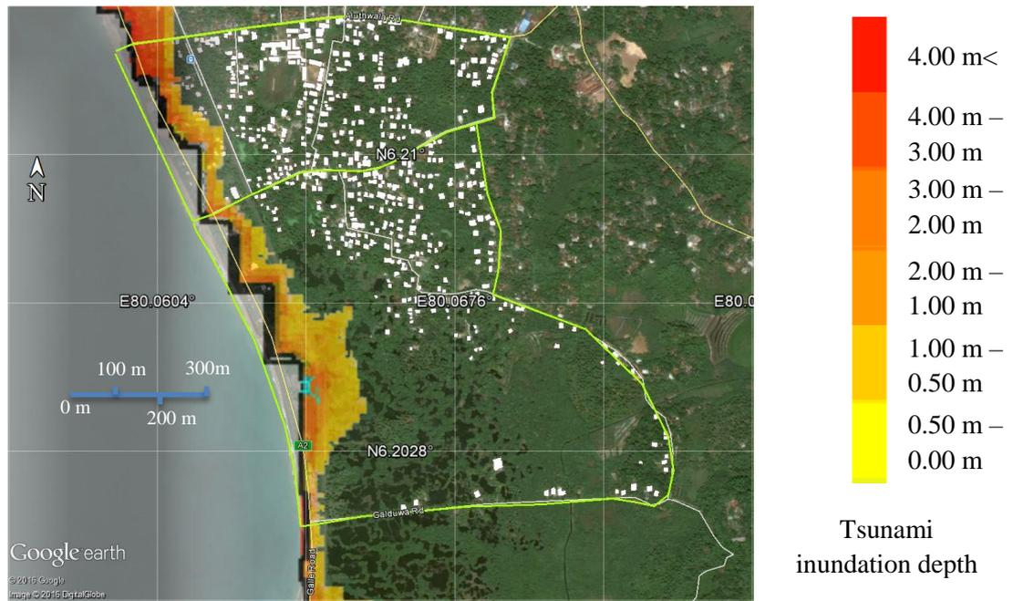
Figure 45: Tsunami inundation depth – Scenario 8 (Mw = 9.0)
