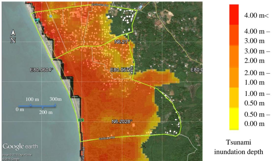
Figure 53: Tsunami inundation depth – Scenario 6 (Mw = 9.0)
