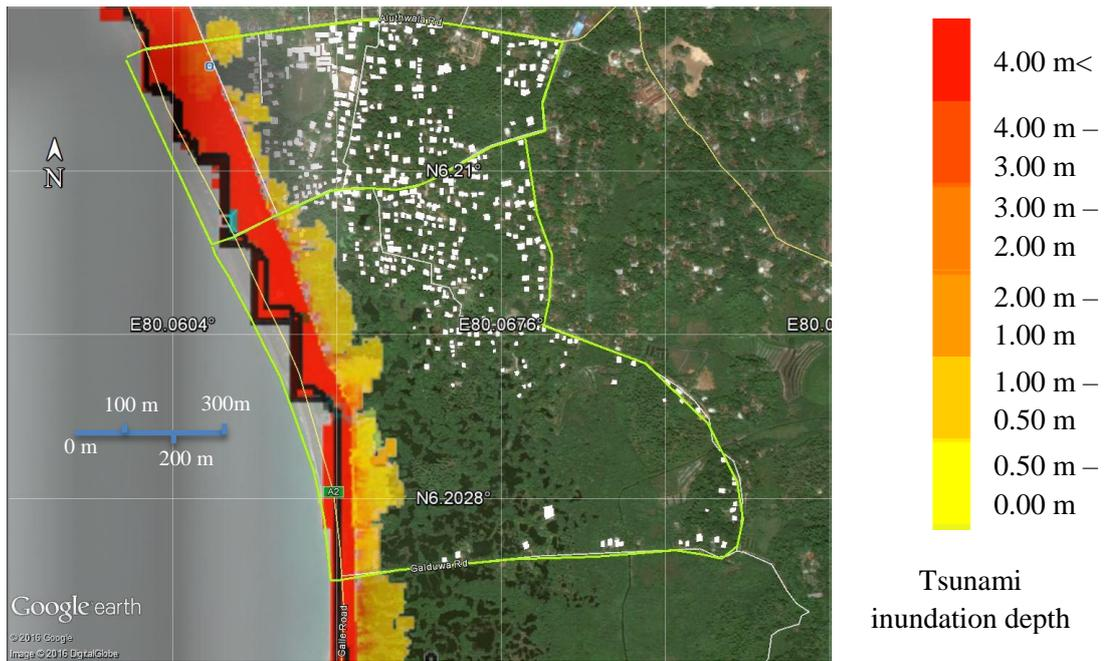
Figure 34: Tsunami inundation depth – Scenario 3 (Mw = 9.1)
