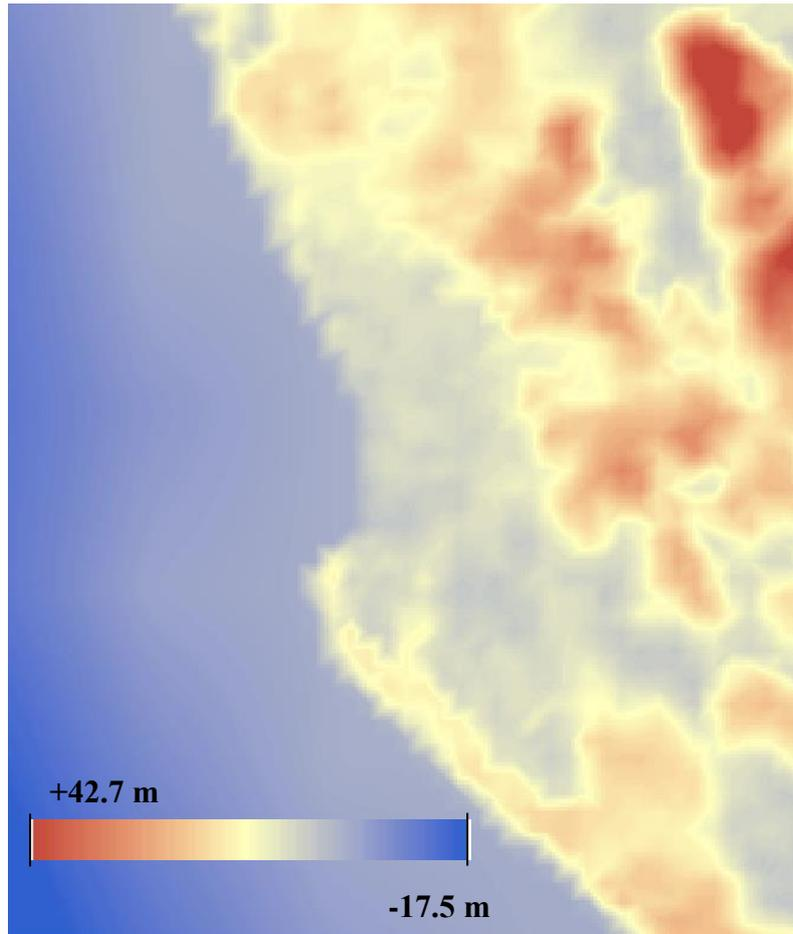
Figure 107: DEM (Digital Elevation Model) (Opened using Arc GIS- Raster (Created using 2385 Points))
