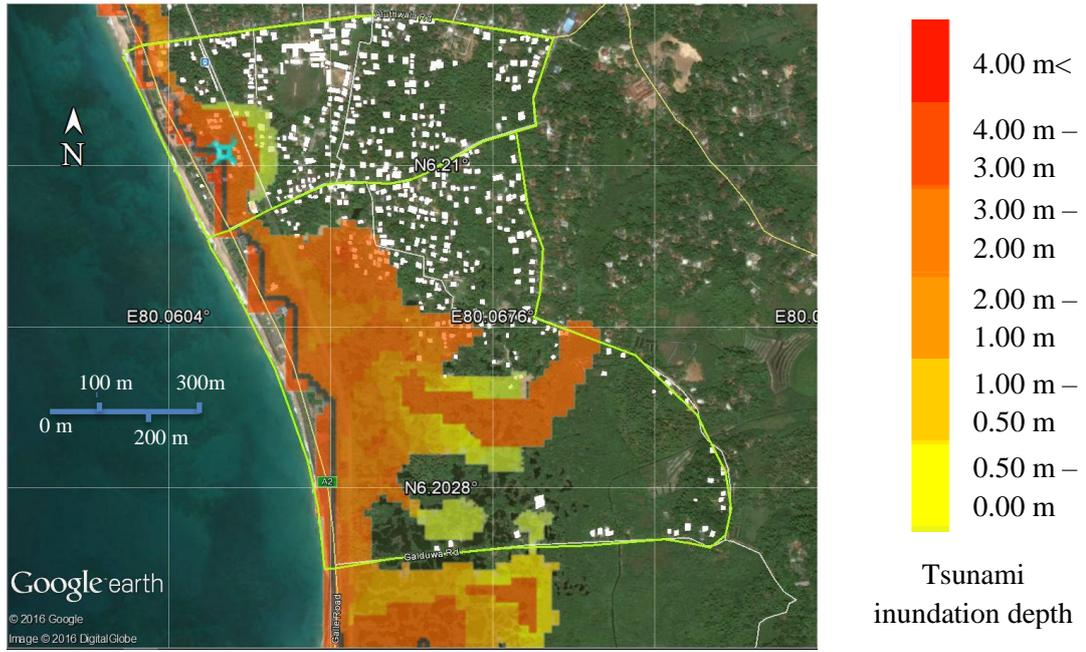
Figure 21: Tsunami inundation depth – Scenario 1 (Mw = 8.8)
