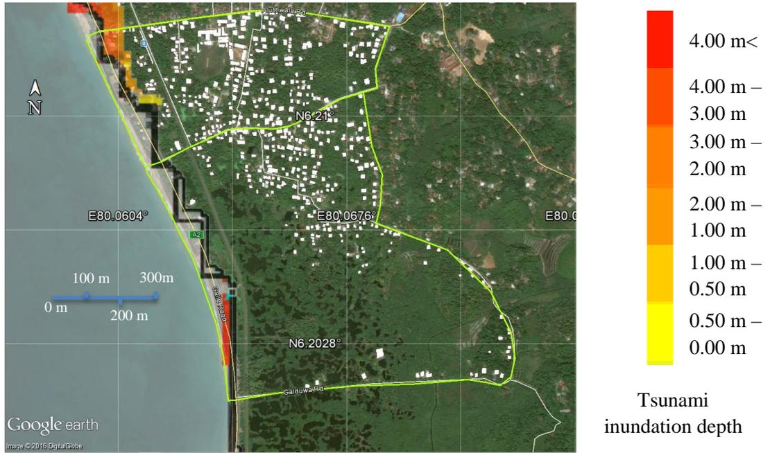
Figure 52: Tsunami inundation depth – Scenario 10 (Mw = 8.9)
