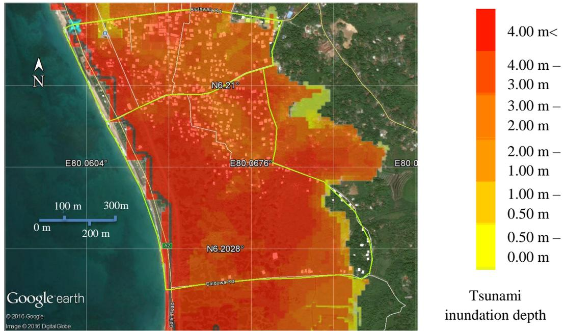
Figure 24: Tsunami inundation depth – Scenario 1 (Mw = 9.1)
