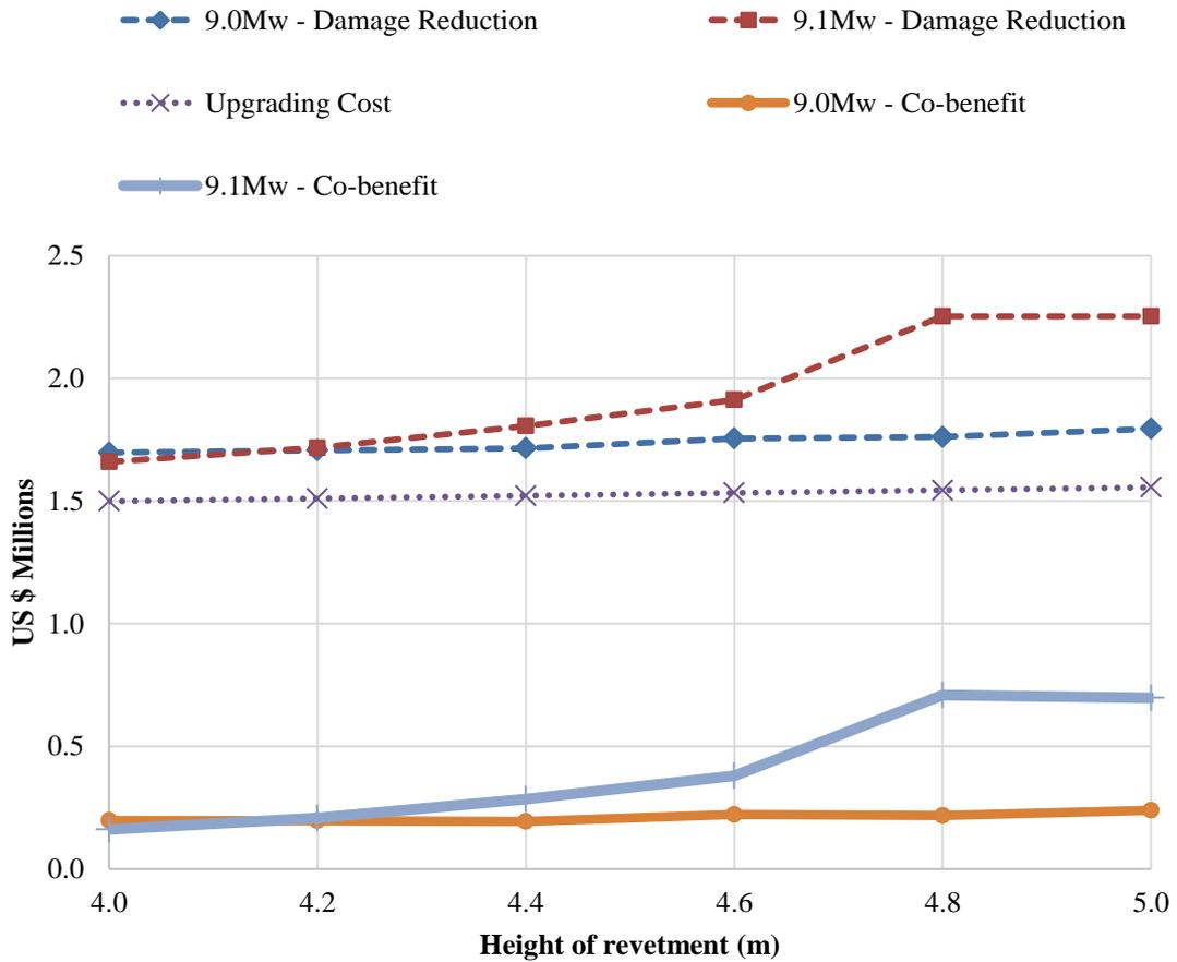
Figure 100: Tsunami co-benefit vs. height of revetment
