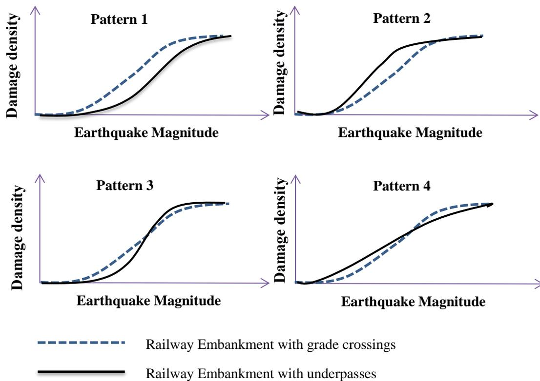
Figure 92: Expected results of damage density vs. earthquake magnitude (Schematic diagram)
