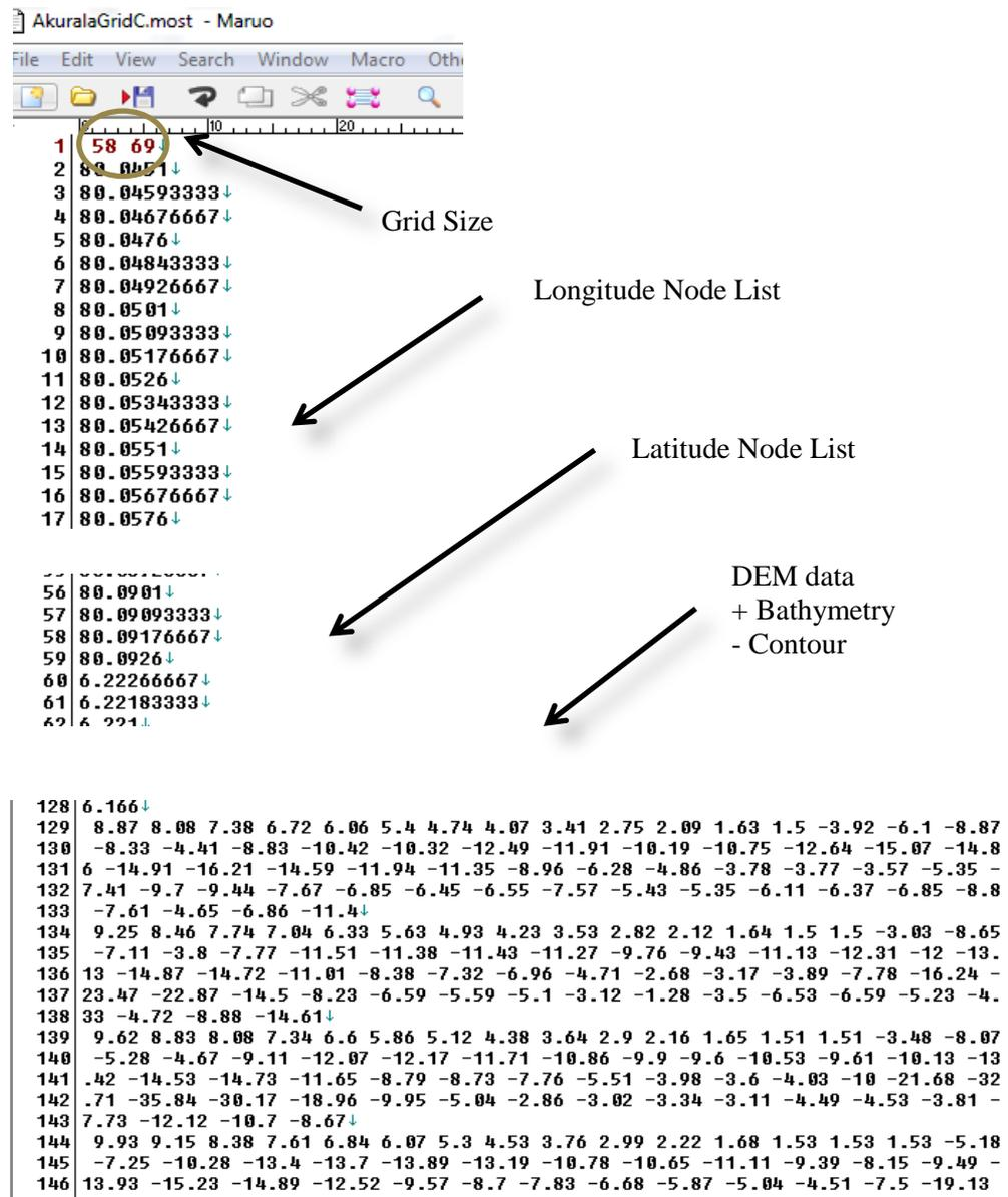
Figure 103: Data format of DEM (Digital Elevation Model) (Opened using Maruo Editor)
