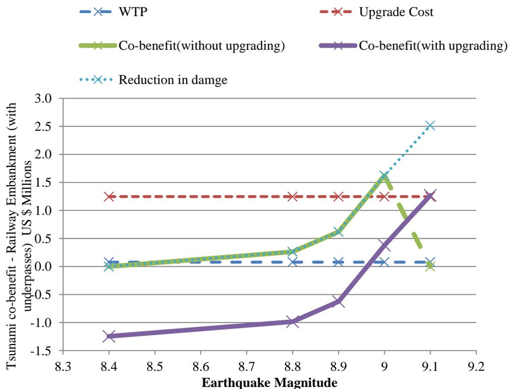
Figure 98: Tsunami co-benefit of railway embankment with underpasses vs. earthquake magnitude
