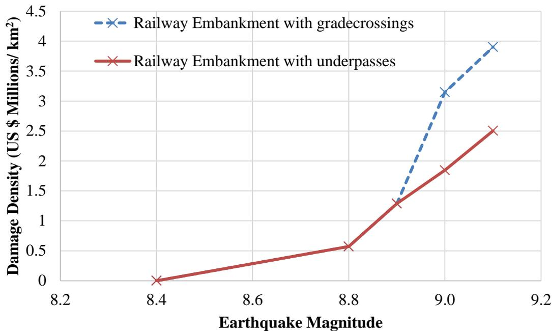
Figure 93: Damage density vs. earthquake magnitude
