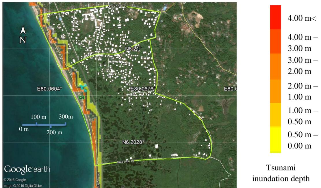
Figure 30: Tsunami inundation depth – Scenario 3 (Mw = 8.4)
