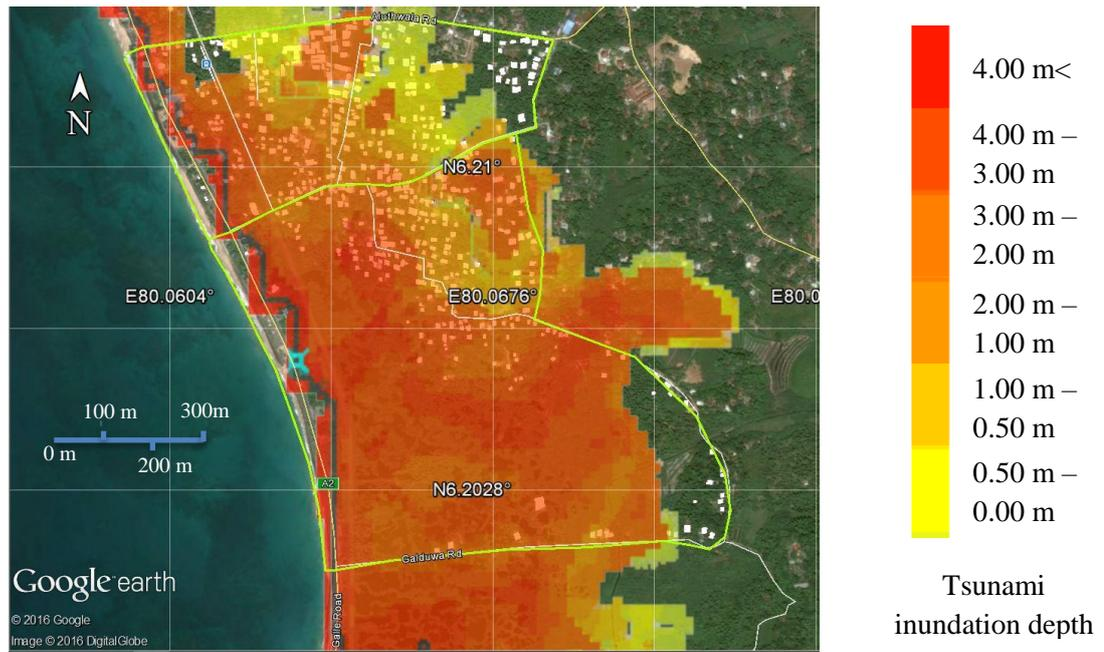
Figure 23: Tsunami inundation depth – Scenario 1 (Mw = 9.0)
