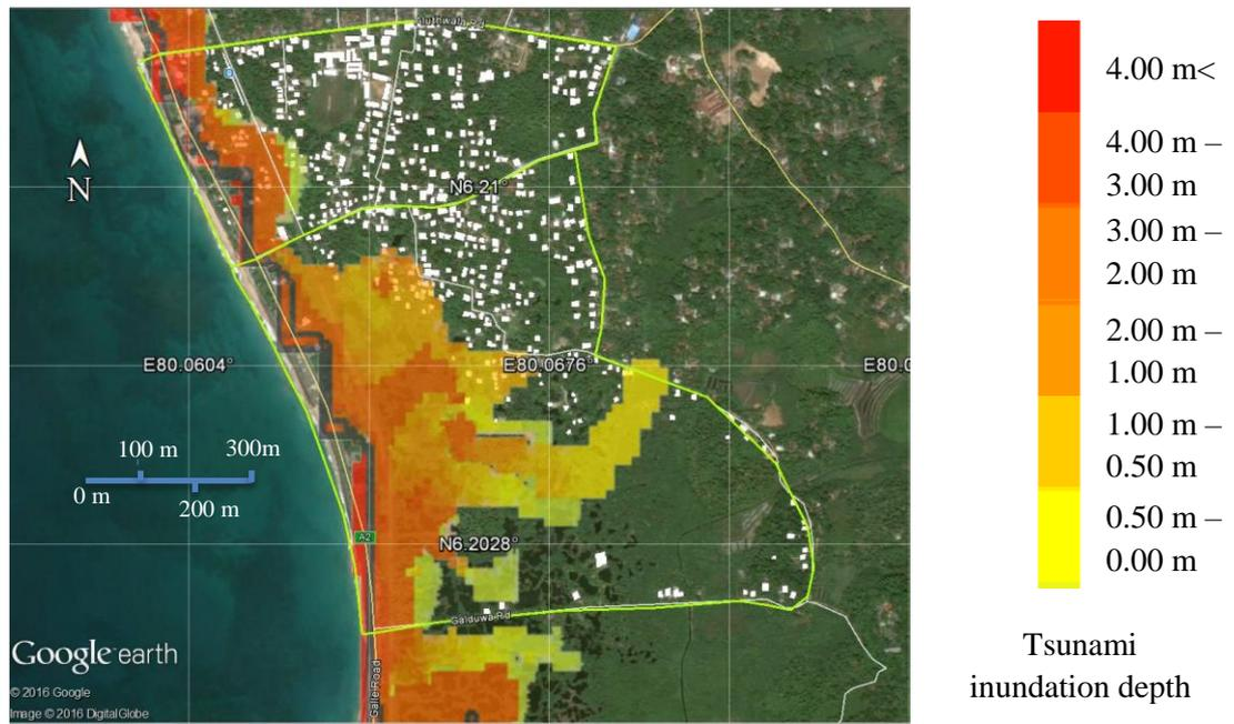
Figure 28: Tsunami inundation depth – Scenario 2 (Mw = 9.0)
