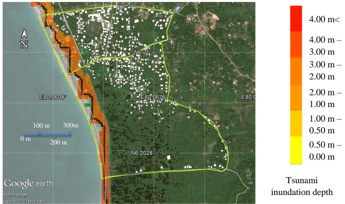
Figure 36: Tsunami inundation depth – Scenario 4 (Mw = 8.8)
