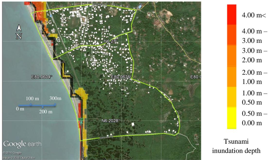
Figure 47: Tsunami inundation depth – Scenario 10 (Mw = 9.0)
