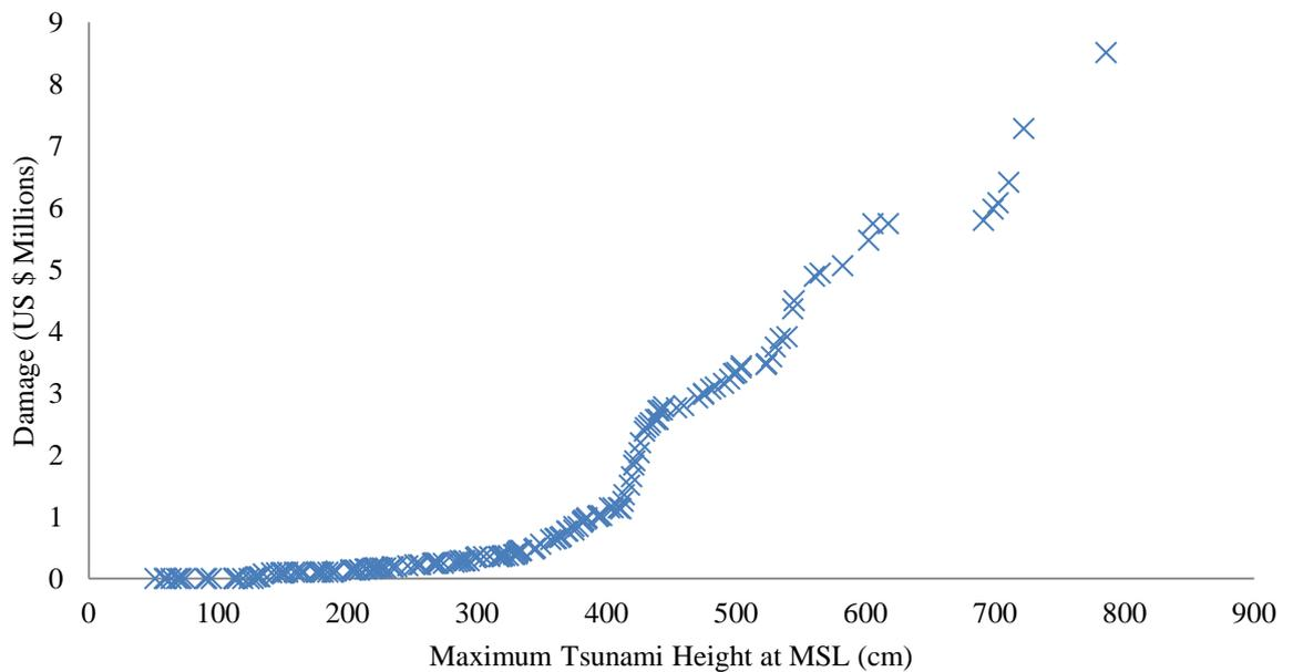
Figure 70: Tsunami damage vs. tsunami height (Without co-beneficial structures)
