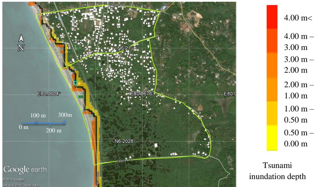
Figure 35: Tsunami inundation depth – Scenario 4 (Mw = 8.4)
