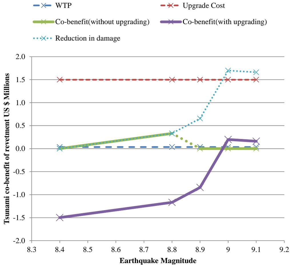
Figure 97: Tsunami co-benefit of revetment vs. earthquake magnitude
