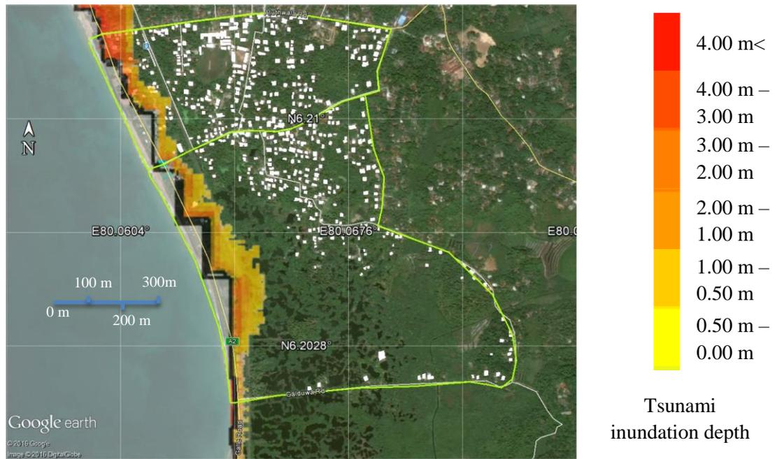
Figure 46: Tsunami inundation depth – Scenario 9 (Mw = 9.0)
