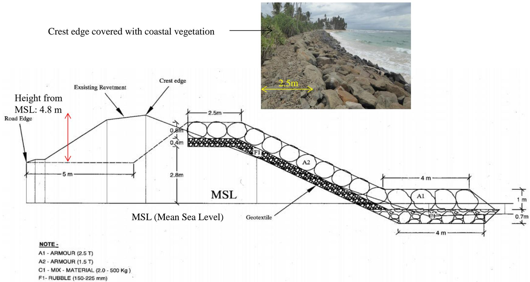
Figure 75: Engineering drawing and a picture of existing revetment in the case study area
