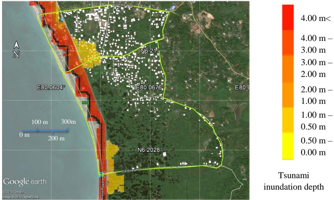
Figure 38: Tsunami inundation depth – Scenario 4 (Mw = 9.0)
