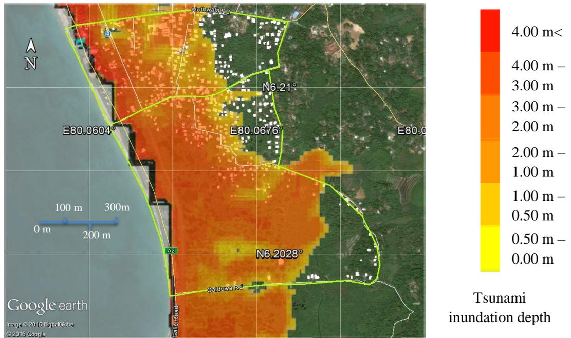
Figure 56: Tsunami inundation depth – Scenario 9 (Mw = 9.0)
