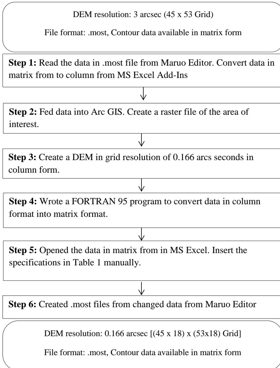
Figure 16: Steps for generating domain C
