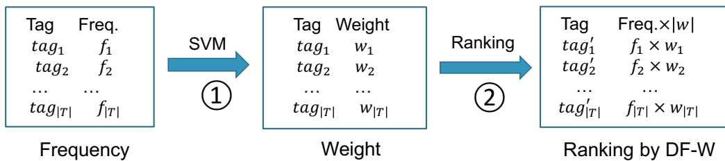
FIGURE 3.1 – The flow of DF-W.
