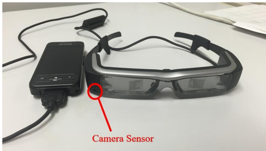
Figure 3.1 EPSON Moverio BT-200 and the position of camera sensor
