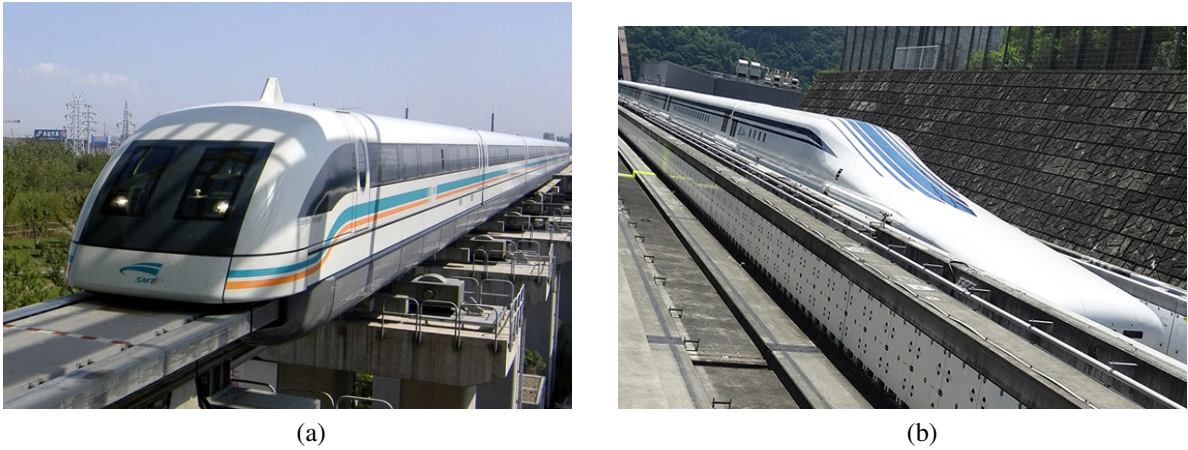
Figure 1.1: (a) Shanghai Maglev based on German EMS Transrapid technology [2]. (b) Superconducting Maglev based on EDS technology in Japan [3].
