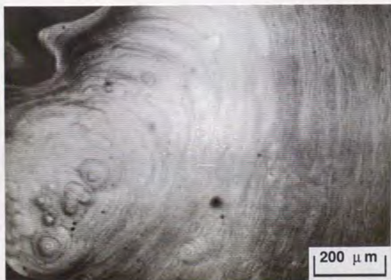
Fig. 5-2. The influence of impurity, GaAs, on morphologies on GaP(111)B surface.
