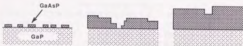
Fig. 2-16. Schematic drawing of morphological changes during GaAsP/GaP growth.
