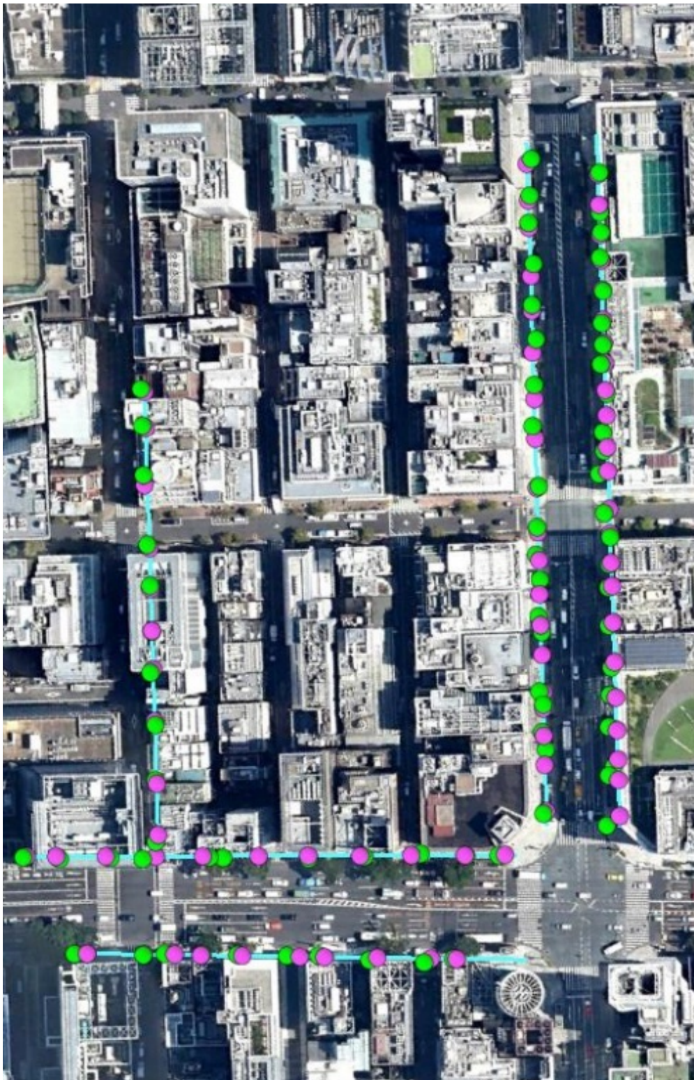
Figure 3.17 Walking trajectory of the experiments in Ginza: walking trajectory (blue line), positioning result (green dot), and ground truth (purple dot)
