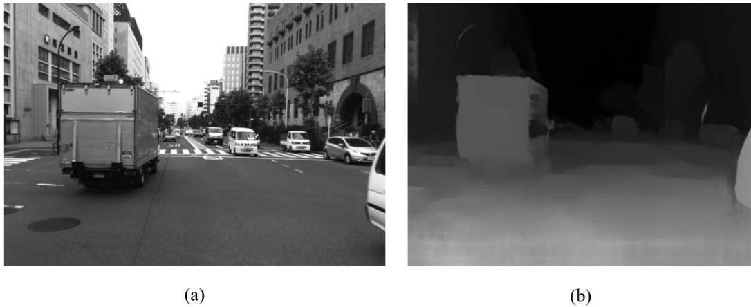
Figure 3.4 Stereo camera images. (a) Image from the left camera; (b) Depth map
