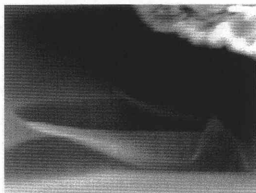
Fig. 4 SEM image of a nano-cantilever after fracture. The point of fracture was at the edge of SiO 2 column.
