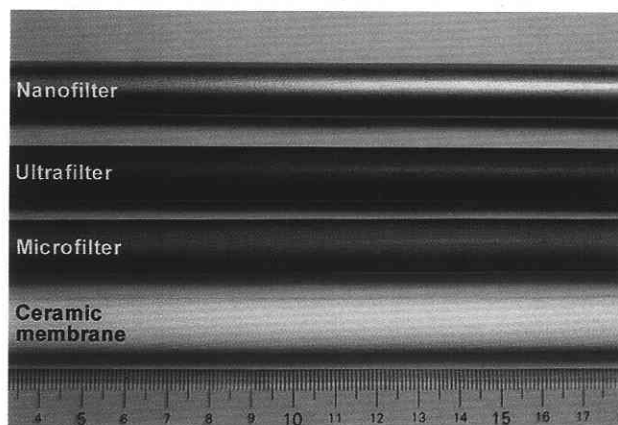
Fig. 1 Carbon coated ceramic membranes by chemical vapor deposition.
