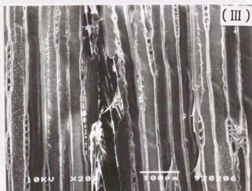
Fig. 7-3. Typical fracture process of the TL system (Spruce, t=120\mu\text{m} ).
