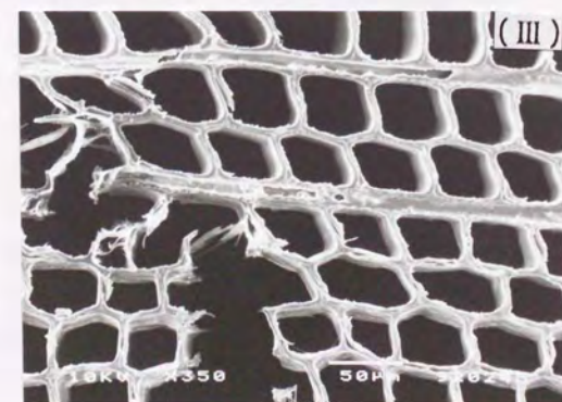
Fig. 7-23. Typical fracture process of the RT system (Spruce, t=120\mu\text{m} ).
