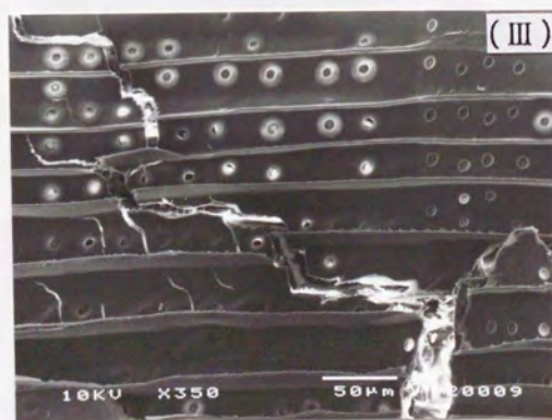
Fig. 7-13. The fracture process of the LR system (Hinoki, t=120\mu\text{m} ).
