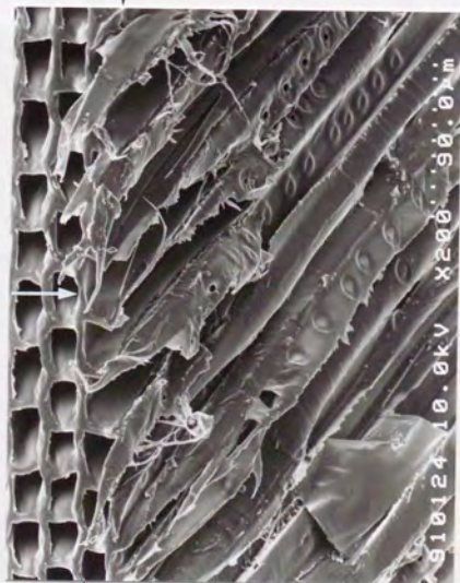
Fig. 5-10. Typical fracture surfaces close to the initial crack tip for the grain angles of 30° and 45°
