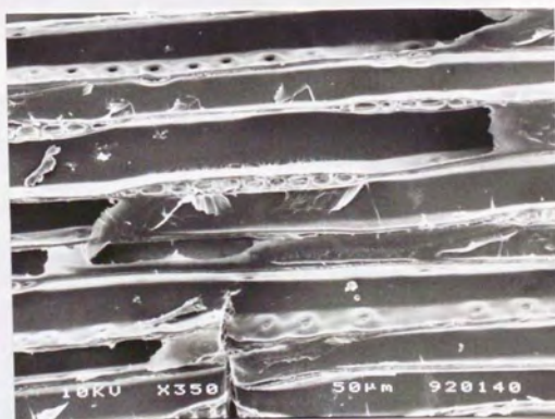
Fig. 7-15. The fracture process of the LT system (Spruce, t=120\mu\text{m} ).
