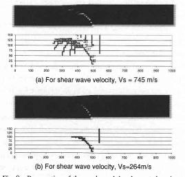
Fig. 9 Propagation of the cracks and the elements location
