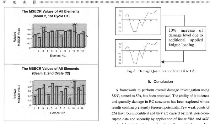
Fig. 6 Damage Localization for Beam 2
