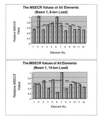
Fig. 5 Damage Localization for Beam 1.
