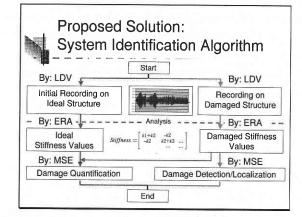
Fig. 1 System Identification Algorithm (SIA) for performing overall damage investigation.
