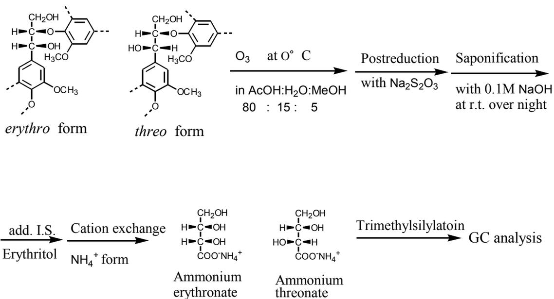
**Fig. 2.1** Experimental scheme for the modified ozonation method
