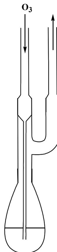
**Fig. 2.2 Reaction vessel**
