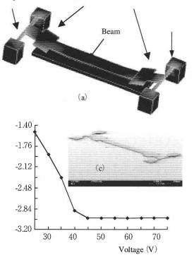
Fig. 6 IEMN Switch with reduced voltage actuation.. (a) Schematic view during actuation. (b) Simulated displacement/voltage characteristic. (c) SEM view of first prototypes.
