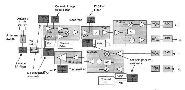
Fig. 1 System-level schematic of a superheterodyne transceiver front-end architecture<sup>5</sup>.
