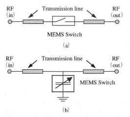
passes through the coplanar waveguide (pass-through state). When an electrostatic voltage (typically 50V) is applied between the membrane and the bottom (signal) electrode, the membrane is pulled down onto the dielectric layer. The coupling capacitance between the signal line and the grounded membrane increases (impedance to ground decreases) and thus blocks the RF signal from passing through to the other side of the signal line.
