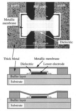
Fig. 5 Capacitive coupling switch developed by Raytheon/Texas Instrument<sup>17-18</sup>. (a) Micrograph. (b) Schematic cross sectional view.
