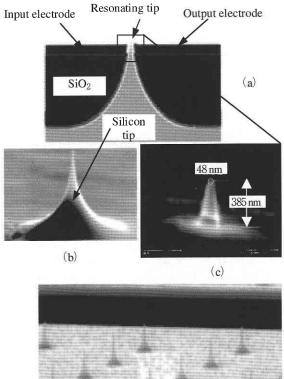
Fig. 3 RF electromechanical resonator based on vibrating tips<sup>24</sup>. (a) Principle. (b) Sharpened silicon tip. (c) resonating tip apex after inter-tip area filled with SiO<sub>2</sub>. (d) Array of tips before SiO<sub>2</sub> filling.
