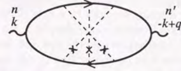
Fig. 28 Maximal crossed diagram giving a weak localization correction to the Boltzmann conductivity.
