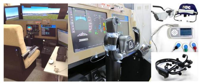
Fig. 4. Simulator of the Suzuki-Tsuchiya laboratory at The University of Tokyo. Left: overview. Middle: Sternberg 7 digits secondary task and response switches (Yellow & Orange) attached to the control column. Part of the primary flight display is covered for experiment's primary task purposes. Right: Eye mark camera, Portable ECG device, and brainwave measurement headset.
