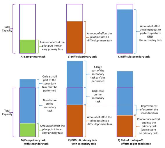
Fig. 1. Illustration of how a difficult secondary task can be used to measure the amount of effort a subject puts into the primary task, assuming the single channel capacity model.
