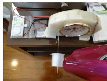
Fig.4. Rotating Savonius turbine (December 12, 2011)
