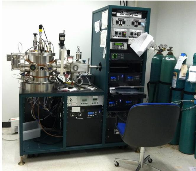
**Fig. 2.4** ATC Orion sputtering system (from AJA International, Inc.) used for depositions of thin film electrolytes and electrodes.
