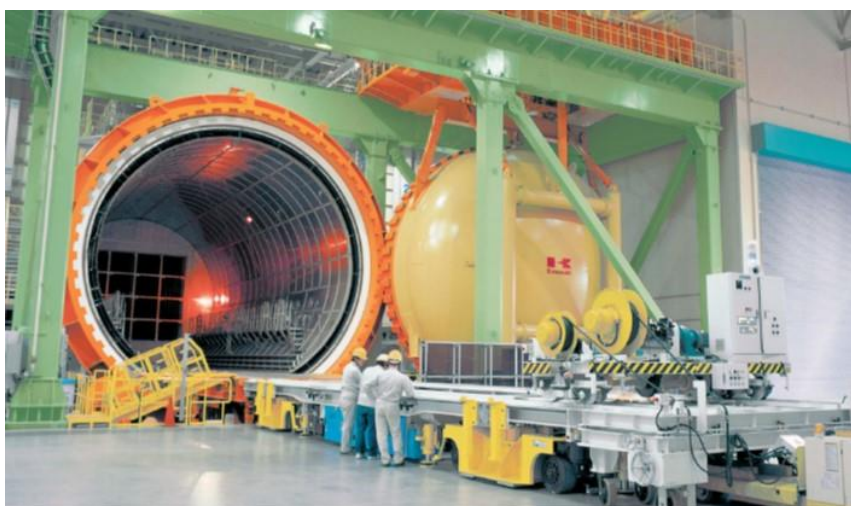
Fig.1.7 Autoclave for airplane produced by Kawasaki heavy industries[13].
