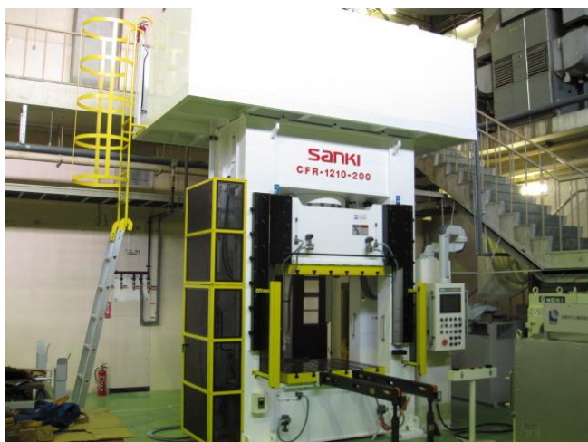
Fig.E.18 Hydraulic press for stamp molding (2000 kN).
