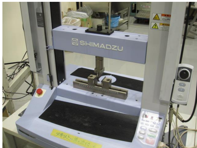
Fig.E.7 Test machine and bending set-up.
