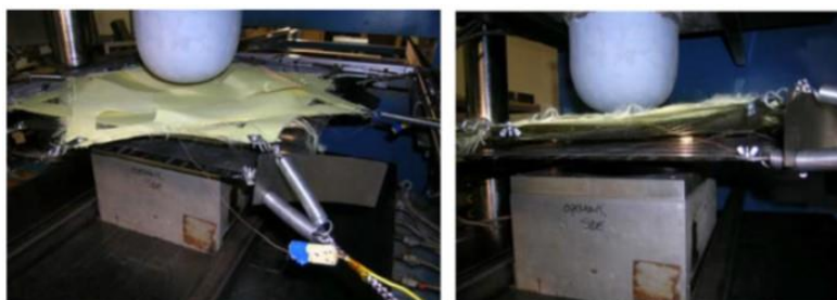
Fig.4.9 Stamp molding of consolidated blank with tension [101].
