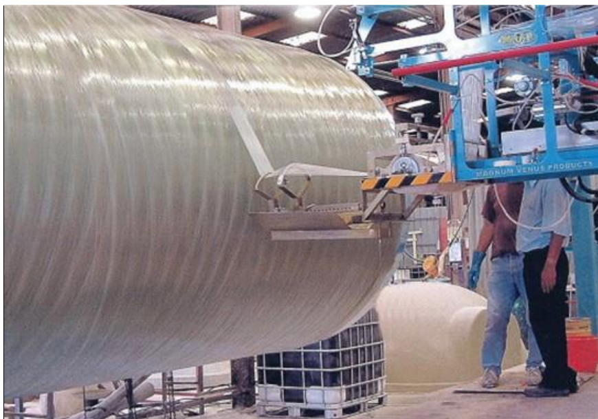
Fig.1.11 Glass fiber composite pipe by filament winding [34].
