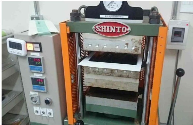
Fig.E.3 Double platen hot and cold press (100 kN).
