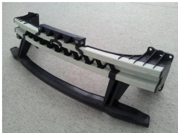
Fig.4.14 Front bumper beam produced by curved reactive thermoplastic pultrusion [107].
