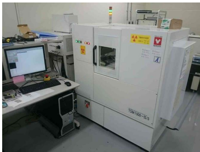
Fig.E.10 X-ray 3D microscopic CT scanner.
