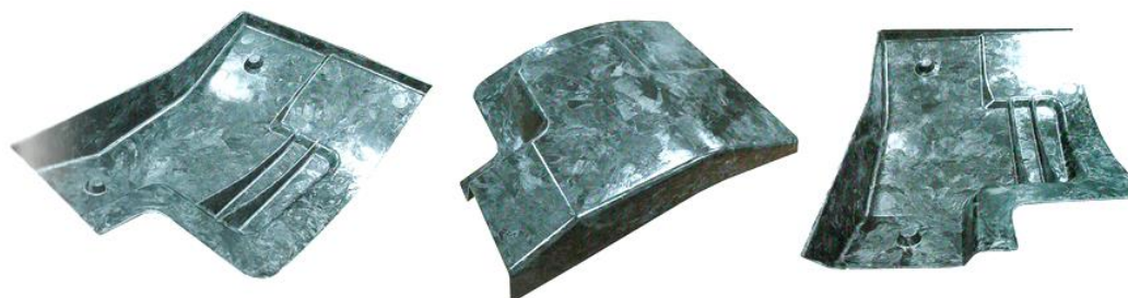
(b): Molding products made of CF-SMC
