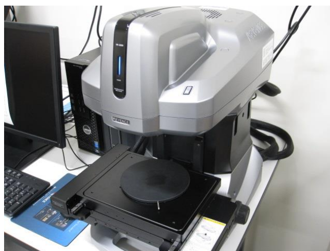
Fig.E.11 Laser 3D measurement microscope.
