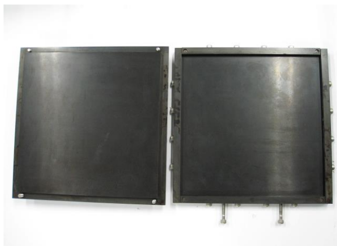
Fig.E.2 Steel mold for making 200-200 mm composite plate.
