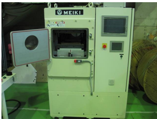
Fig.E.20 Vacuum press preheater (400 kN).
