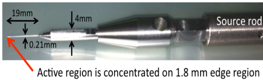
Figure 7.3: ^{57}\text{Co} calibration source rod
