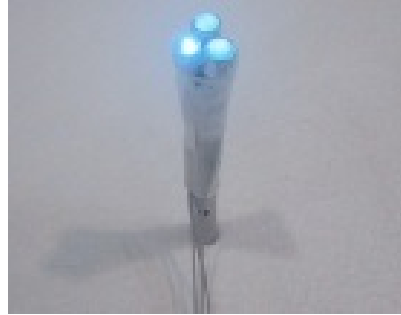
(b) LED for the gain calibration. Three LEDs of different intensities are bundled.
