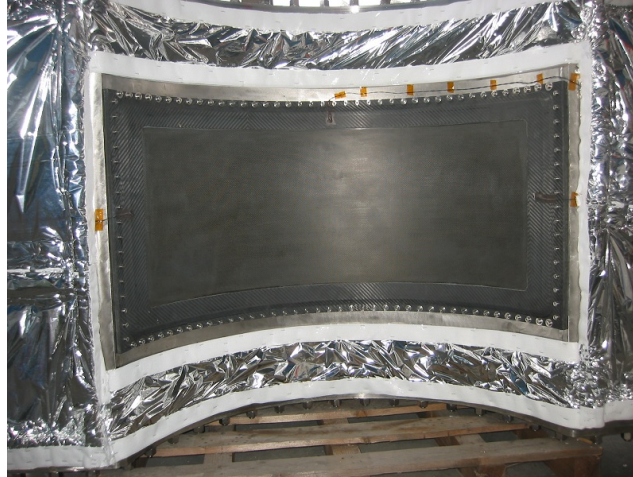
Figure 2.12: Honeycomb panel is attached on the entrance window of inner vessel. The panel has a dimension of 1315 \times 611\text{mm}^2 along curved inside face.
